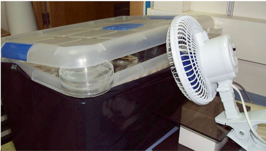
Fig. 9.12 The partially opened incubating cooler with a fan for ventilation
