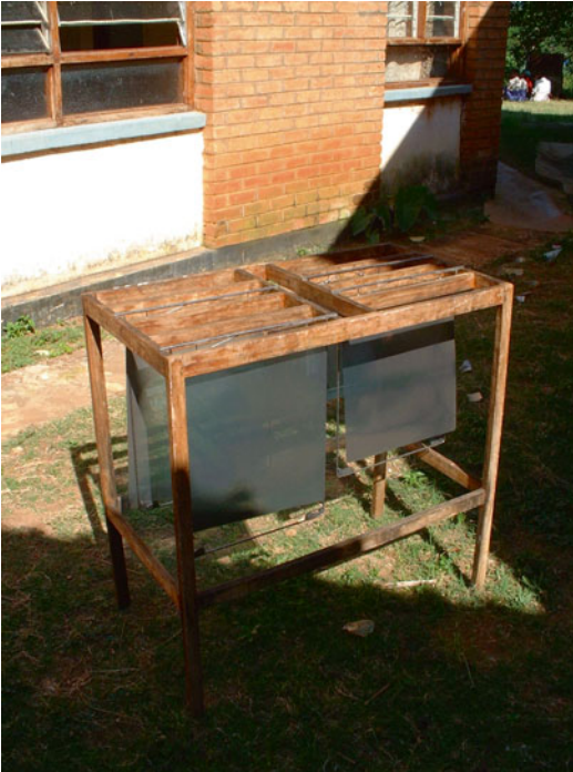
Fig. 23.4 Rack for drying films outside
