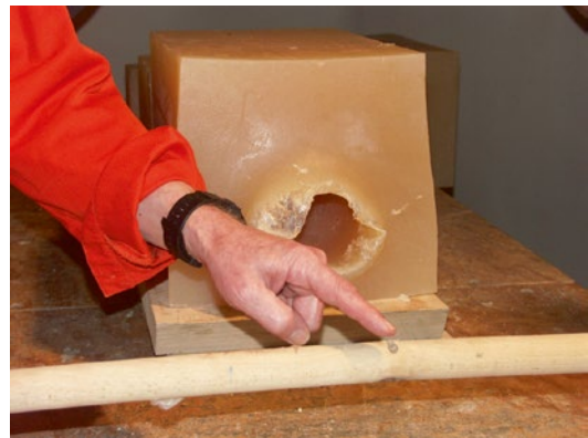
Fig. 8.4 Ricochet effect (Swiss Army Ballistic Laboratory in Thun, Switzerland. ICRC war surgery seminar, 2005). A 7.62×51 fmj bullet (same as in lower blocks of 38–1) has been destabilized just before impact by placing a wooden broomstick along its flight path (note the small nick on the stick) resulting in a sideway impact of the bullet with a resulting almost instant transfer of energy totally different from the lower blocks profile in Fig. 9.3. This phenomenon is actually quite common in real cases when bullets are fired through vegetation or hit walls or ground before the final human target
