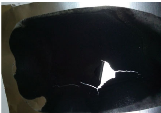
Fig. 1 Poor adhesion of 75:5:20 composition with substrate, getting peeled off from surface after drying
