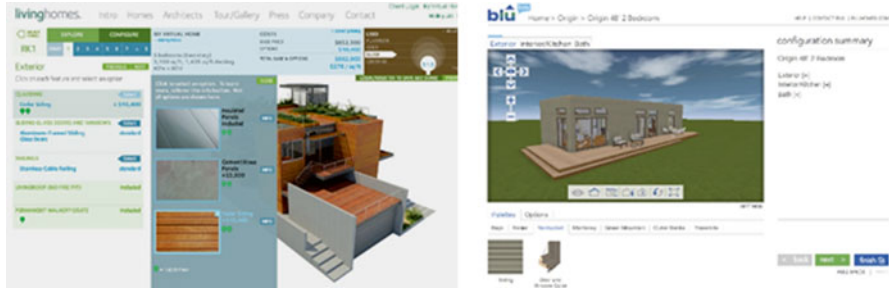
Fig. 5.1 Screenshots from configuration system by LivingHomes and Blu Homes, consecutively. The process has high visualization qualities in both cases, where LivingHomes utilize static images that changes in response to user selection, while Blu Homes employ an interactive 3D configurator plug-in (Source: http://www.livinghomes.net/configure.html?model , http://www.bluhomes.com/homeconfigurator/ )
