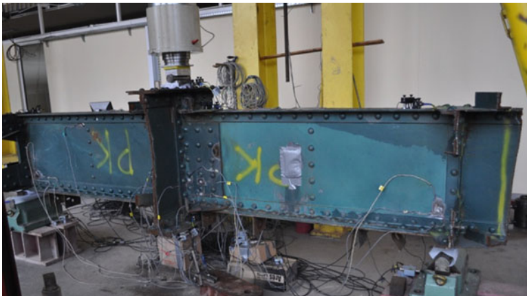
Fig. 5 View of joint on test stand
