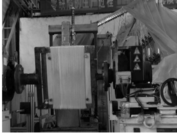
Fig. 2 The reinforced glass fiber-winding process
