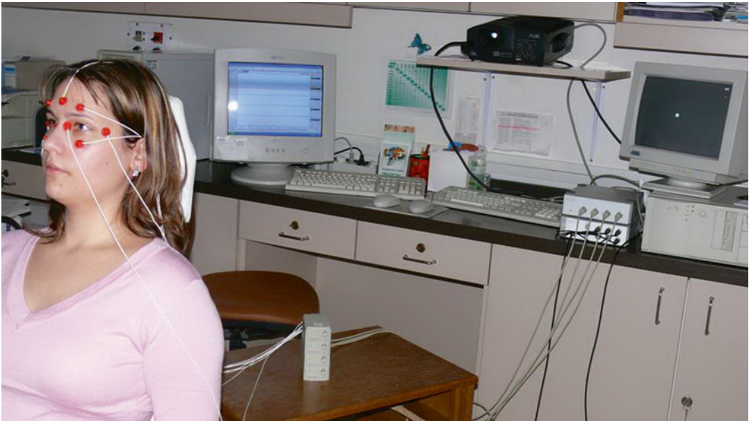
Fig. 33.2 The DC recorder, the collector head connecting to the amplifier device and the computer are behind the examined subject
