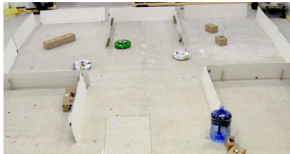
(b) The robot in depot 1 sees a large box, so it turns on the red light (the light is not shown).
