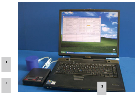
Fig. 7 Thermal biosensor system based on the principle of the measurement of the heat transferring and the solid phase electrolyte thermistors. 1—thermal sensitive unit; 2—interface with the registration unit; 3—laptop
