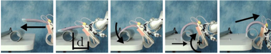
Fig. 13 Edge grasp with the RBO hand, from left to right approach, compliant contact with the edge, sliding object along surface, sliding fingers along surface, and lift
