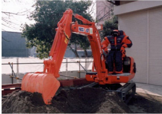
Fig. 2 Tele-operated HRP-1S driving the backhoe
