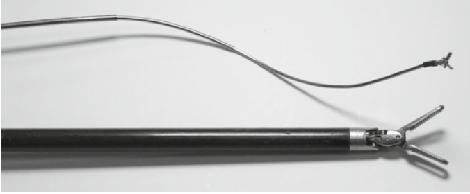
Fig. 1 A concentric tube robot next to a standard da Vinci laparoscopic tool
