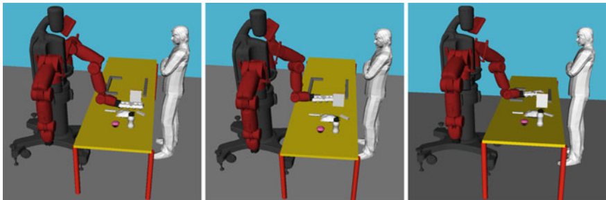
Fig. 11 Shows the learned trajectory for moving an egg carton. Since eggs are fragile robot moves the carton near the table surface. (Left) Start of trajectory. (Middle) Intermediate waypoint with egg close to the table surface. (Right) End of trajectory
