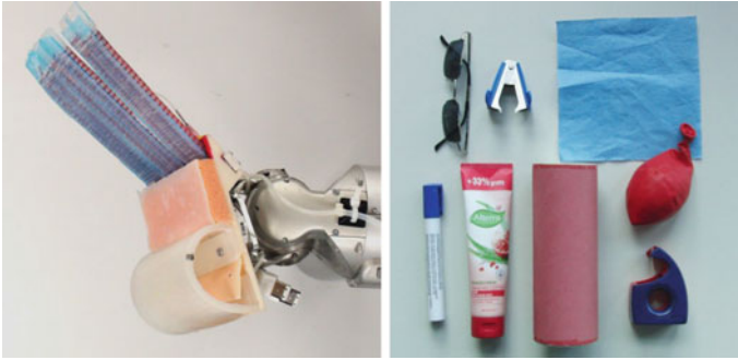
Fig. 10 RBO hand and a selection of objects it can grasp
