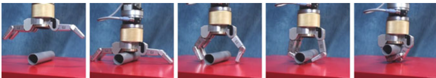
Fig. 5 Force-compliant closing strategy, from left to right positioning using visual feedback, contacting table surface using force feedback, closing fingers using position feedback while wrist is force-compliant in z -direction (last three images)
