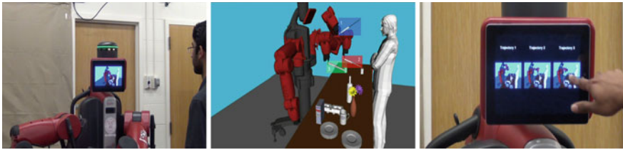
Fig. 2 Re-rank feedback mechanism: (Left) Robot ranks trajectories using the score function and (Middle) displays top three trajectories on a touch screen device (iPad here). (Right) As feedback, the user improves the ranking by selecting the third trajectory
