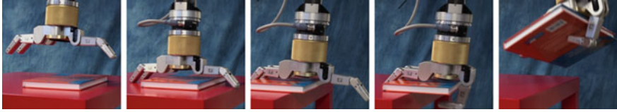
Fig. 7 Slide-to-edge grasp strategy, from left to right positioning using visual feedback, contact surface using force feedback, moving towards the edge while being force-compliant in the z -direction of the wrist, closing the thumb when the hand is above the edge (detected via visual feedback), and lifting
