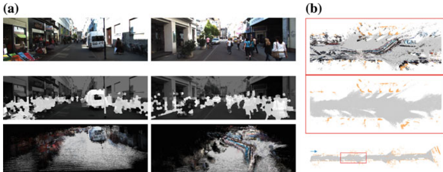
Fig. 5 Segmentation by our recursive inference process in a high dynamic street in downtown. a A couple of frames with the highlighted objects class. b Reprojected point cloud for the ground and building class, on the top we show also the objects class
