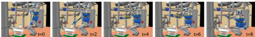
Fig. 11 Reaching motion executed by the left arm . The robot lowers its body to avoid its left shoulder colliding with a pipe [8]
