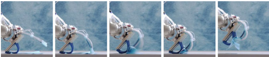
Fig. 12 Surface constrained grasp picking up a piece of tissue, from left to right exploitation of table to position and orient the hand, exploitation of table to ensure contact with the flat object, compliant grasping, established grasp, and object lift
