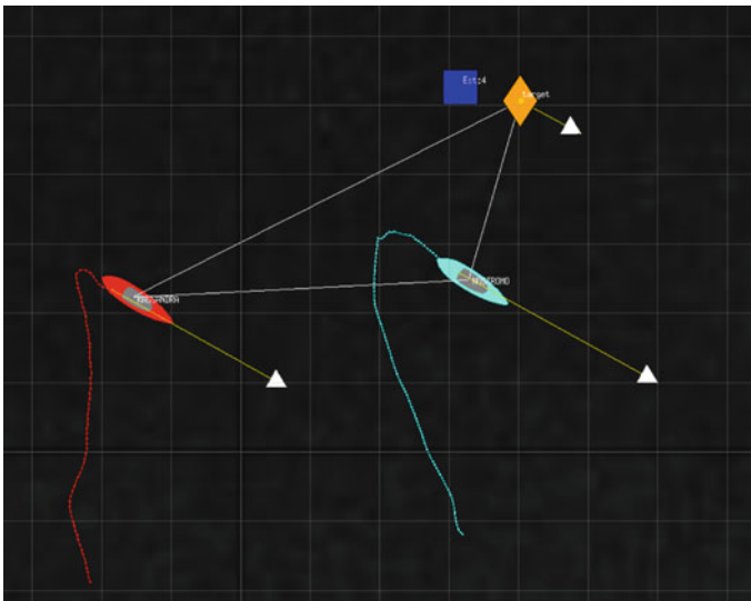
Fig. 1 Screenshot from an active localization and pursuit experiment with acoustic communications. The two vehicles jointly estimate the target location based on range measurements, and move to stay in formation relative to it
