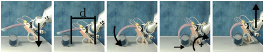
Fig. 11 Execution of a surface-constrained grasp, from left to right approach phase, exploitation of table to position and orient the hand, the fingers pull the object across the constraint surface, compliance achieves large contact area, and object lift
