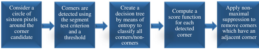
Fig. 7 The main steps of the FAST corner detector [22]
