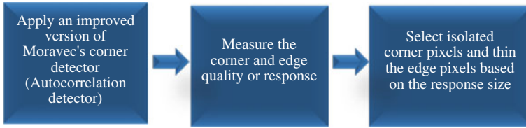
Fig. 5 The main steps of the Harris corner and edge detector [19]
