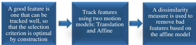
Fig. 10 The main steps of the GFTT corner detector [10]
