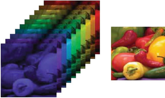
Fig. 1 An illustration of the spectral data with ten bands and the corresponding image as it would be acquired with a color imager [3]
