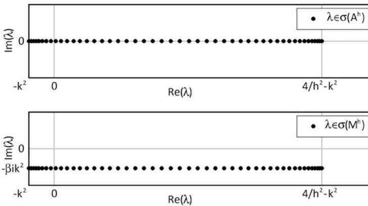
Fig. 1 Top : spectrum of the 1D Helmholtz operator discretized using second order finite differences on a 48 \times 48 equidistant grid with standard homogeneous Dirichlet boundary conditions. Bottom : spectrum of the corresponding Complex Shifted Laplacian (CSL) operator
