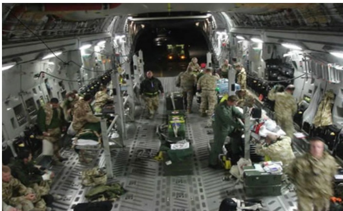
FIGURE 19.2 A Royal Air Force C17 in aeromedical configuration. The patient at the far right rear of the aircraft is ventilated. The other patients are of a lower dependency. The ambulance is visible just beyond the open ramp. Medical lacons are stropped centrally for ease of access with black roll bags containing consumables hanging at the side (Reproduced with permission: Sgt Chris Andrews, Tactical Medical Wing, RAF Brize Norton)
