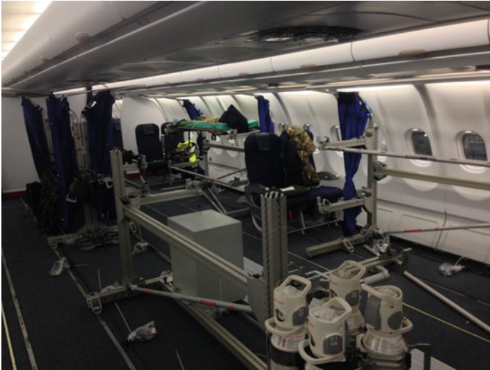
FIGURE 19.3 The stretcher stanchions on the RAF Voyager aircraft (Airbus A330-200). The oxygen cylinders can be seen secured at the head end. This central stanchion is designed for critical care patients with all round access. Some of the stretcher fits in the background have privacy curtains fitted. The seats would be allocated to the AE team
