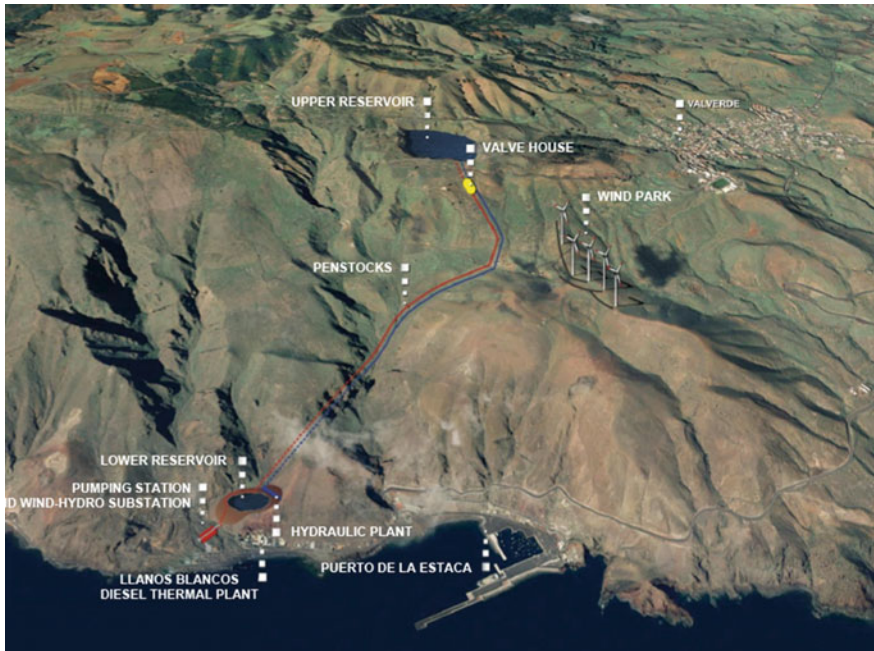
Fig. 8 Wind-pumped hydro generation plant, coupled with a previous diesel plant, in El Hierro (Gorona del Viento S.A. 2014, with permission)
