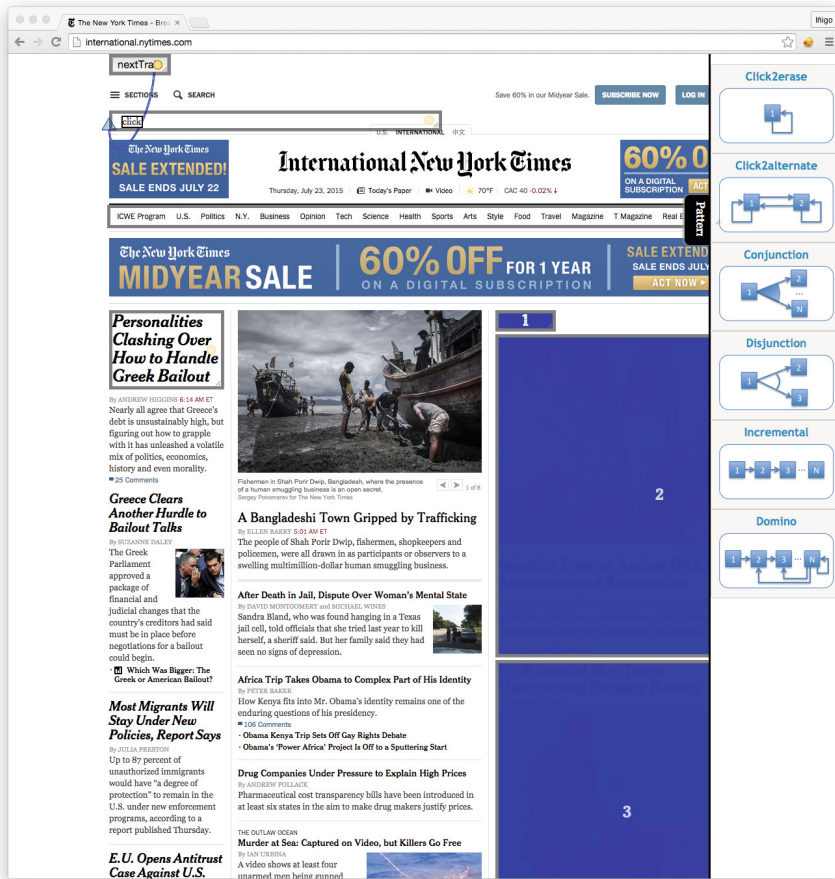
Fig. 8. Setting patterns. Keeping the ALT key pressed down, select first the widgets, and next, the blink pattern.
