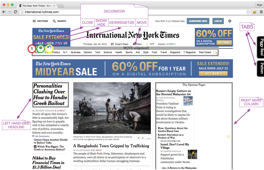
Fig. 3. DOM nodes are turned into widgets. A decorator permits to operate upon the widget: remove, visibility-state modification and un-widgetization (i.e. turning back to a mere DOM node).
