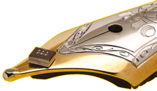
Fig. 15.1 Photograph of a miniature chip-scale packaged (CSP) MEMS resonator including an integrated temperature sensor and heater for calibration with dimensions of 1.5 mm × 1.1 mm × 0.5 mm
