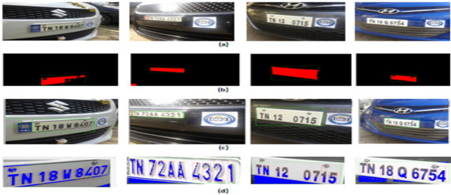
Fig. 6 Real time autonomous license plate extraction and recognition inclined at 30° (a) Original image, (b) Color thresholding at 30° left/right, (c) Localization of plate at 30° left/right, (d) OCR over number plate at 30° left/right
