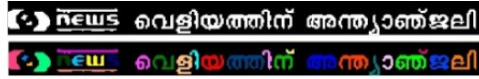
Fig. 4 Ticker text extracted from a news video frame and corresponding connected components
