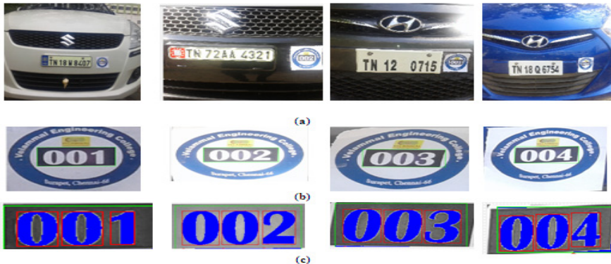
Fig. 5 Real time autonomous sticker number extraction and recognition. (a) Original image, (b) sticker number localization, (c) segmentation and shape extraction
