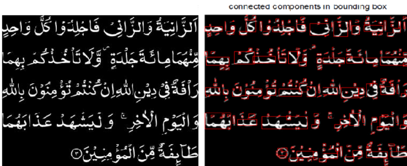
Fig. 3 Identification of objects in an Arabic document image shown in left. Connected components are enclosed in rectangle(red color)
