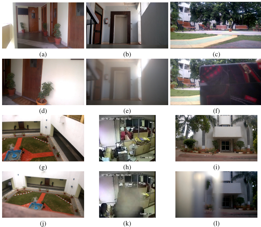
Fig. 1 Example frames showing camera tamper. (a), (b), (c), (g), (h) and (i) are the original intended camera scene images, (d) view after camera displacement (e) view after camera defocus (f) obstructed view by placing object in front of camera (j) view after camera displacement (k) view after camera defocus and (l) obstructed view by placing object in front of camera
