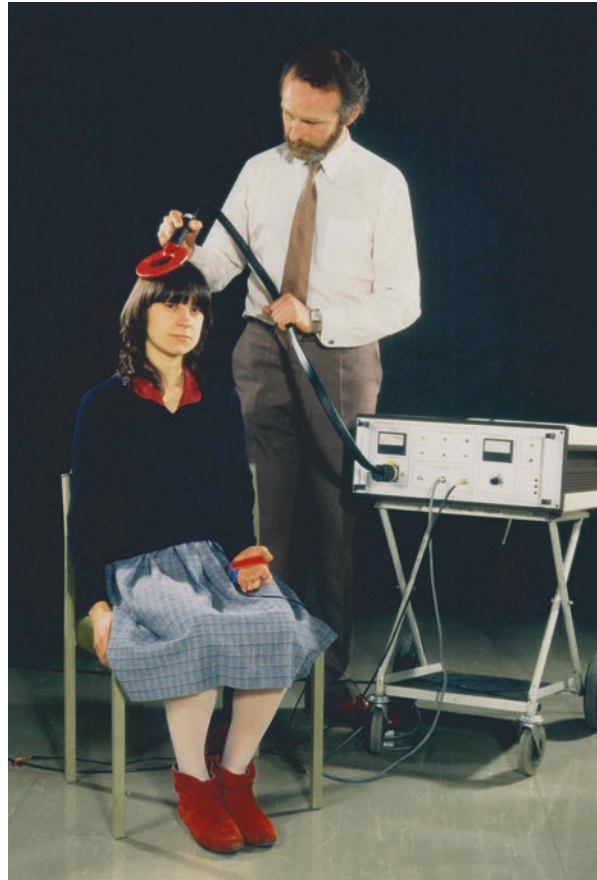
Fig. 6.3 The first repetitive transcranial magnetic stimulation (rTMS) system developed in Sheffield, UK (With permission from Professor A. Barker)
