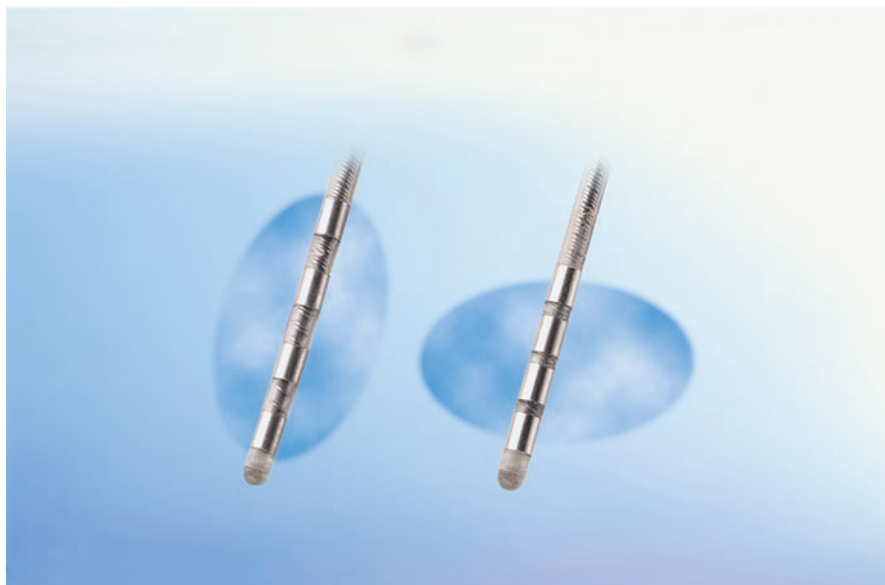
Fig. 5.1 The quadripolar electrodes (leads) used for deep brain stimulation. Each contact on the electrode is 1.5 mm long and 1.27 mm in diameter. On the left is model 3387 (produced by Medtronic), in which the contacts are spaced 1.5 mm apart. On the right is model 3389, in which the contacts are spaced 0.5 mm apart (Reprinted with the permission of Medtronic, Inc. © 2014)
