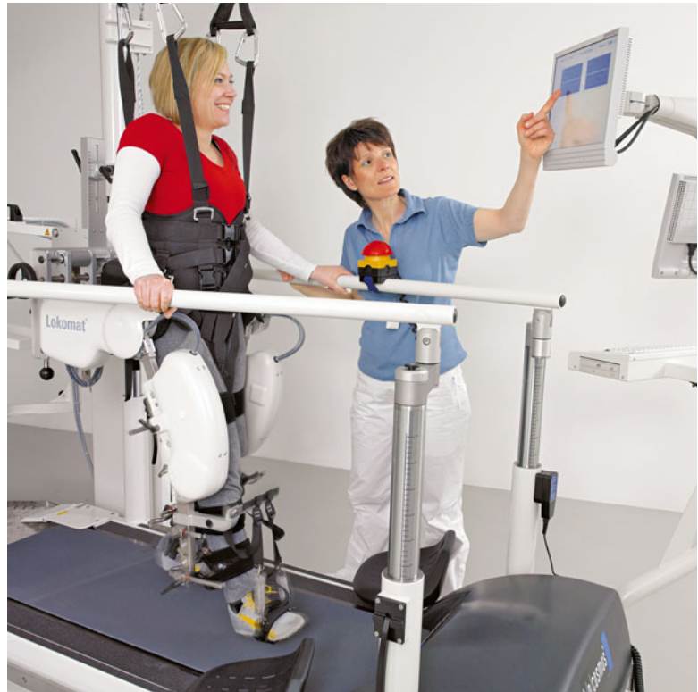
Fig. 12.1 Exoskeletal systems like the Lokomat (Hocoma AG, Switzerland) apply exoskeletons that move the patient's legs in the sagittal plane in conjunction with a body weight support system
