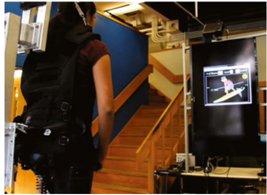
Fig. 20.9 View from the MIT-Skywalker. A large screen is used to display games and real-time webcam video of the subject
