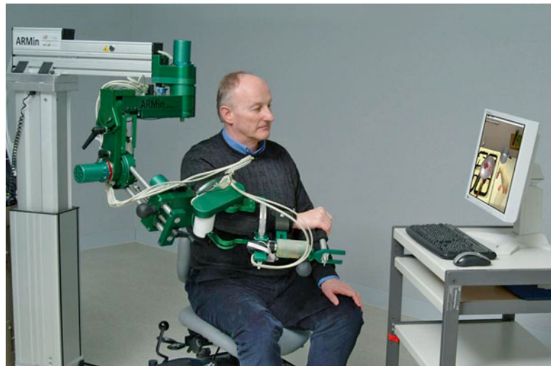
Fig. 17.3 ARMin I robot with a healthy test person ( left ). The person is looking at a computer monitor showing the movement task ( right )
