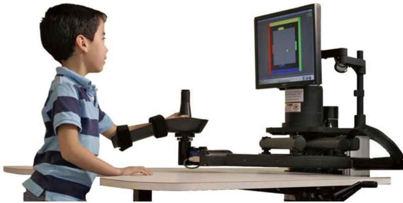
Fig. 14.6 The upper extremity end-effector device InMotion2 (Interactive Motion Technologies, Watertown, MA, USA) allows to train planar movements in a two-dimensional workspace. This device is nowadays
