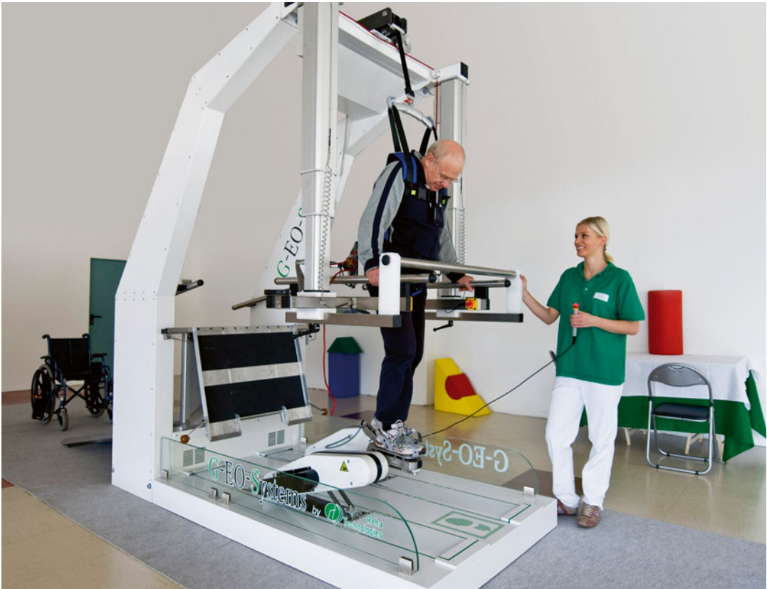
Fig. 12.2 End-effector-based systems like G-EO systems (Reha Technologies, Olten, Switzerland) work like conventional elliptical trainers, where the subject's feet are strapped to two footplates moving along a gait-like trajectory
