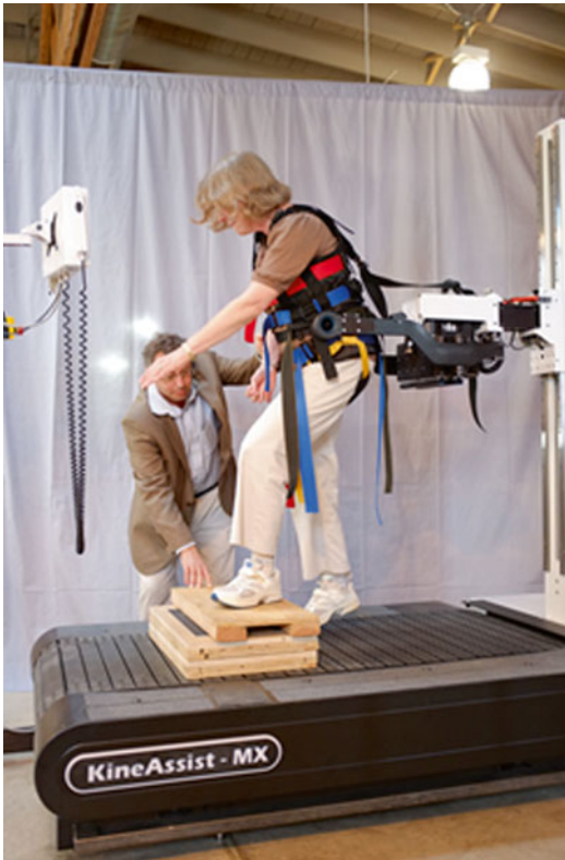
Fig. 3.7 Example of robotic device (KineAssist MX, HDT Robotics) that was used to enable to stroke survivors to practice highly challenging balance and walking tasks while also providing safety and stability against falls. (Photo courtesy of HDT Robotics)
