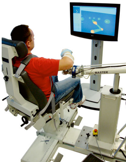
Fig. 18.4 Example of a research participant positioned with the ACT-3D showing the five reaching targets (From Ellis et al. [6]; used with permission)
