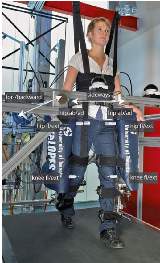
Fig. 22.1 Subject attached in the first prototype of the LOPES device. The eight actuated DOFs are schematically indicated
