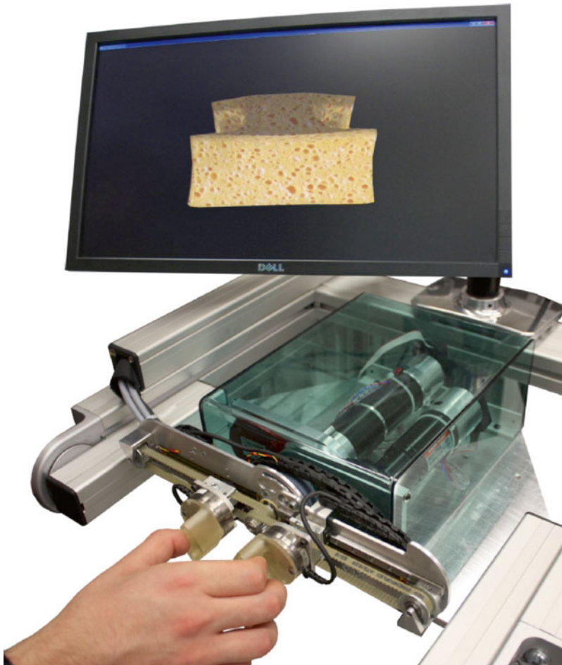
Fig. 15.5 Sample training exercise with a robot designed to provide therapy for sensation. User picks the length corresponding to the virtual object represented by the haptic trainer (Photo courtesy of Dr. Roger Gassert, ETH Zürich)
