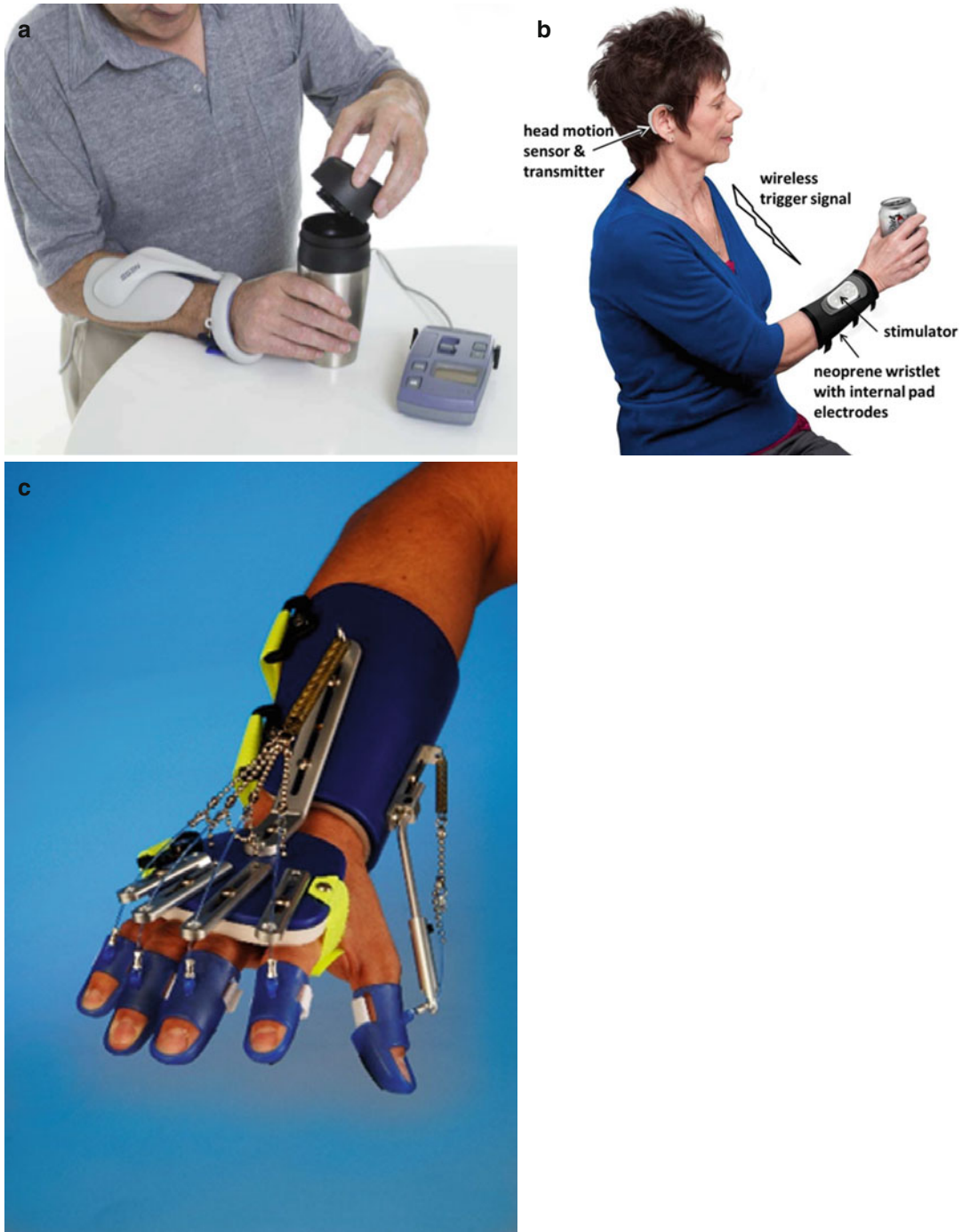
Fig. 26.3 (a) Bioness H200 functional electrical stimulator for hand grasp and release; (b) Rehabtronics Hand Stimulator activated by voluntary head nods detected by a wireless earpiece; (c) the Saeboflex spring-loaded hand-opening splint
