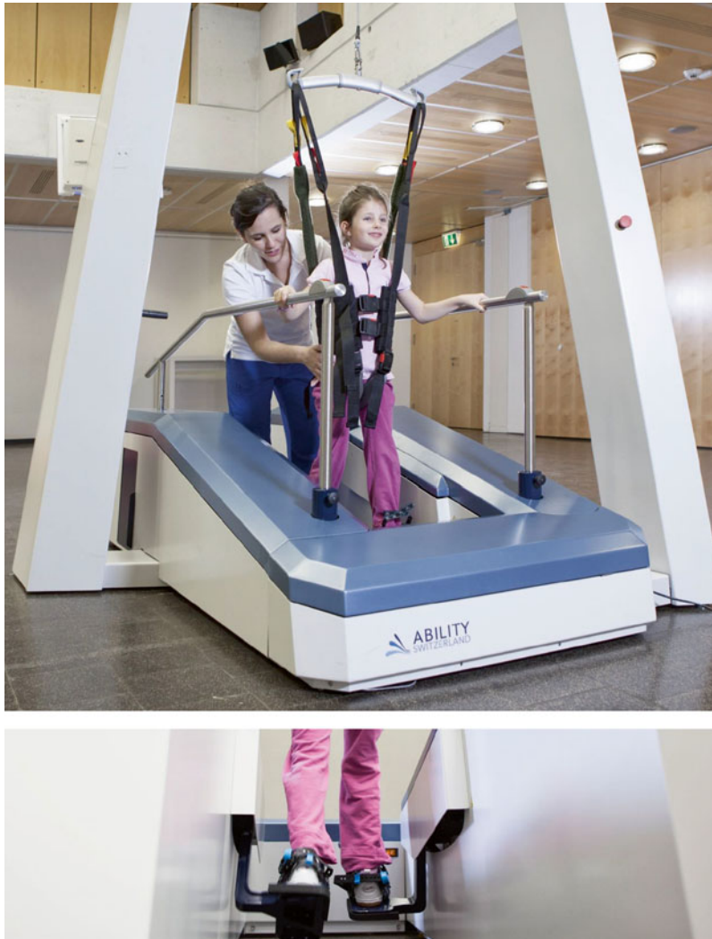
Fig. 14.2 The end-effector gait trainer LYRA (Ability AG, Zurich, Switzerland) allows to train children and youths with body heights varying between 1.00 and 1.95 m and a bodyweight up to 150 kg. The patient is positioned on footplates, and step lengths can easily be adjusted from 39 to 67 cm according to the patient's need.
