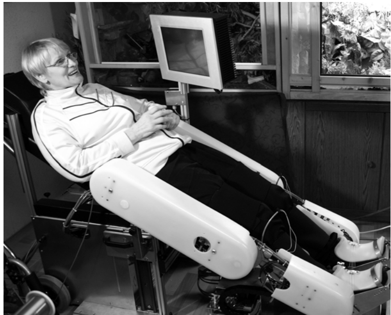
Fig. 8.4 The MoreGait is a pneumatically actuated robot for the training of ambulatory function. The device allows the use at the patient's home
