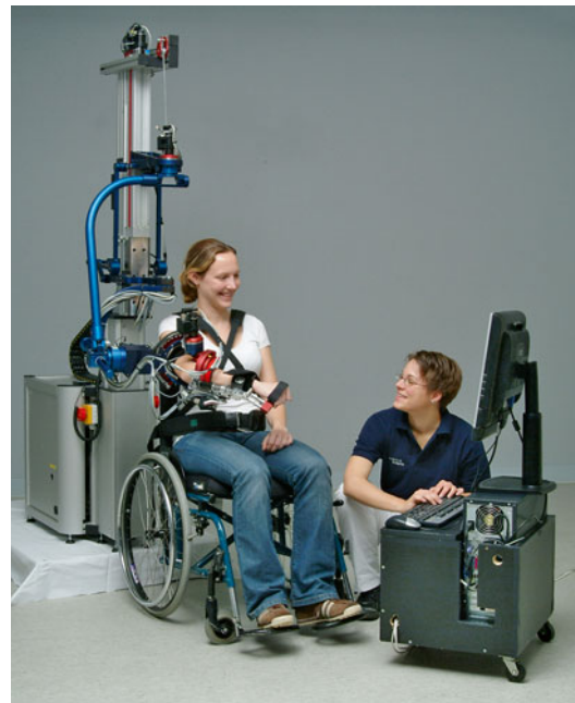
Fig. 17.1 Typical setup for a robot-supported arm therapy system
