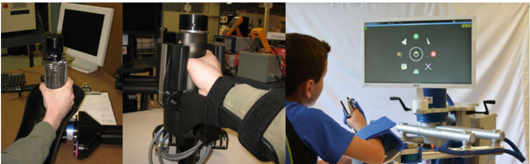
Fig. 16.3 The hand-module evolution. The figure shows the original hand module and several of its commercial variants
