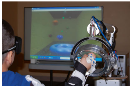
Fig. 28.3 The NJIT-RAVR system utilizes a 3-degree-of-freedom robotic (DOF) interface, the Haptic Master (Moog, The Netherlands), three additional passive DOF via a ring gimbal and a 22-DOF Cyberglove (Cyberglove Systems, USA). The Haptic Master is used to provide haptic rendering of virtual workspaces and adds global forces such as gravity to the virtual environments. The ring gimbal allows for normal positioning of the hand during simulated tasks, and the Cyberglove collects data related to finger position. These interfaces are integrated with a suite of complex, virtually simulated tasks to allow for task-based sensorimotor training for persons with upper extremity hemiparesis [67]
