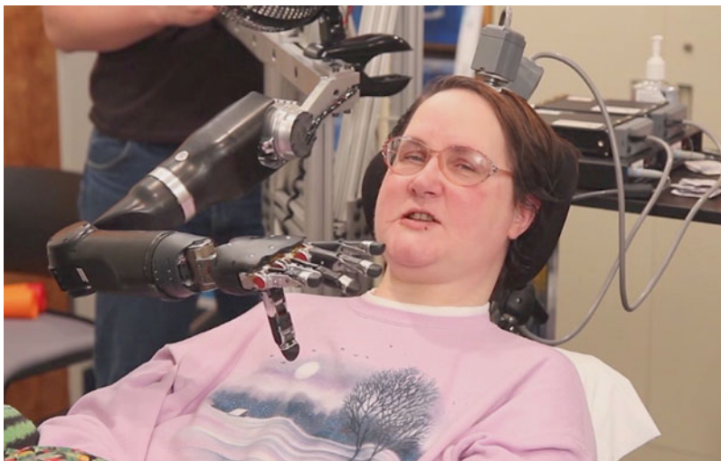
Fig. 15.4 BMI-controlled robotic limbs. Woman with tetraplegia uses modular prosthetic arm to grasp and manipulate objects (Photo courtesy of Motorlab, University of Pittsburgh)
