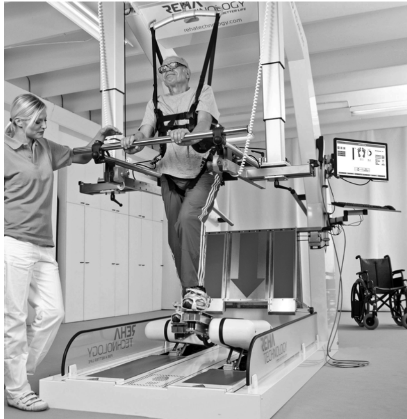
Fig. 8.1 The GEO System assists the patient during gait training using an end-effector-based approach combined with a system for partial unloading of the body weight (Photo courtesy Reha Technology AG, Olten, Switzerland. Used with permission)
