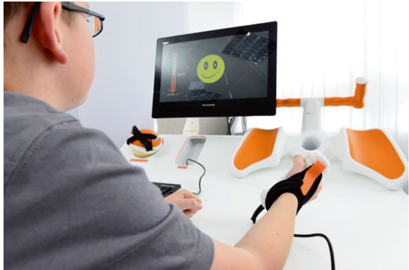
Fig. 14.7 Training elbow and shoulder movements with the Pablo sensor system (Tyromotion GmbH, Graz, Austria). Besides enabling a playful training, the Pablo system is also intended to perform standardized assessments of the upper extremity (Picture with kind permission from Tyromotion)
