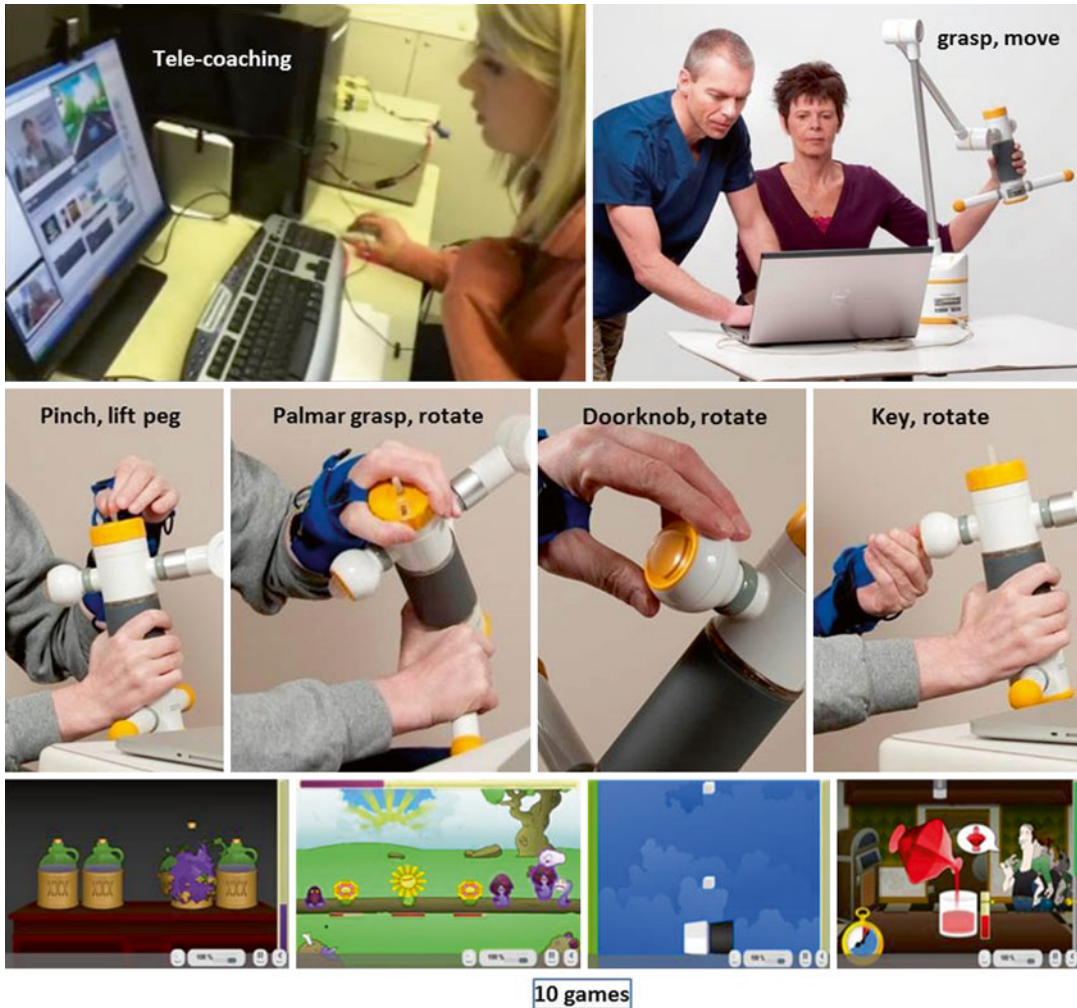
Fig. 26.2 (a) Tele-coaching of an in-home exercise therapy session using the ReJoyce system; (b) participant using ReJoyce workstation to play computer games; (c) movements performed, (d) selected games
