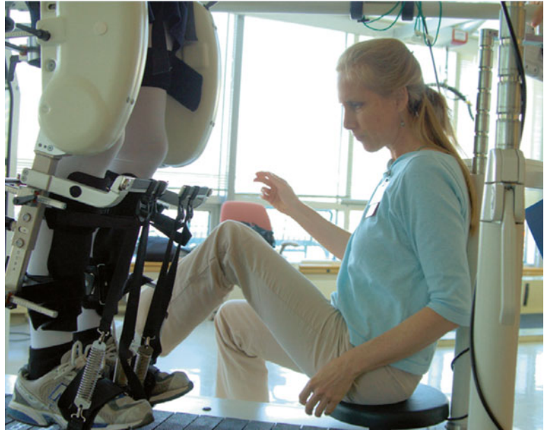
Fig. 12.9 The use of elastic foot lifters is strongly recommended in robotic devices without footplates or boots due to safety reasons as obtaining ankle dorsiflexion for a whole training session will be difficult for most patients (Photo courtesy of Spaulding Rehabilitation Hospital, USA)
