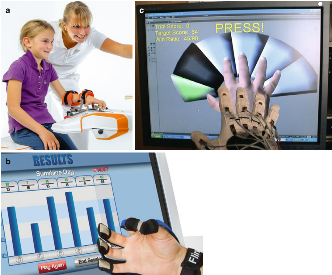
Fig. 15.11 Devices used to train finger individuation. (a) Amadeo (Tyromotion, Inc.) has a separate actuated linear slide for each digit (Photo courtesy of Tyromotion, Inc.). (b) MusicGlove (Flint Rehabilitation) employs sensor in the tips of the digits to detect proper thumb-finger opposition (Photo courtesy of Flint Rehabilitation). (c) The actuated virtual keypad (AVK) employs the PneuGlove with its pneumatically driven air chambers to facilitate practice playing the virtual keypad (From Thielbar et al. [86]; used with permission)
