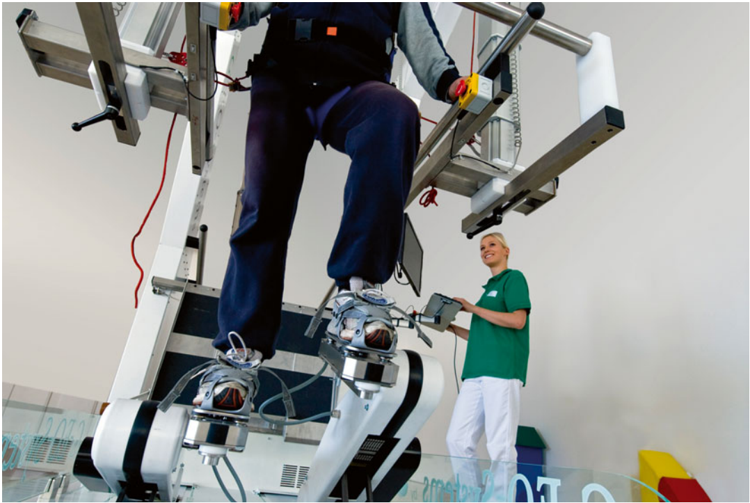
Fig. 12.10 The G-EO systems (Reha Technologies, Olten, Switzerland) allow training of additional tasks, for example, repetitive practice of stair climbing
