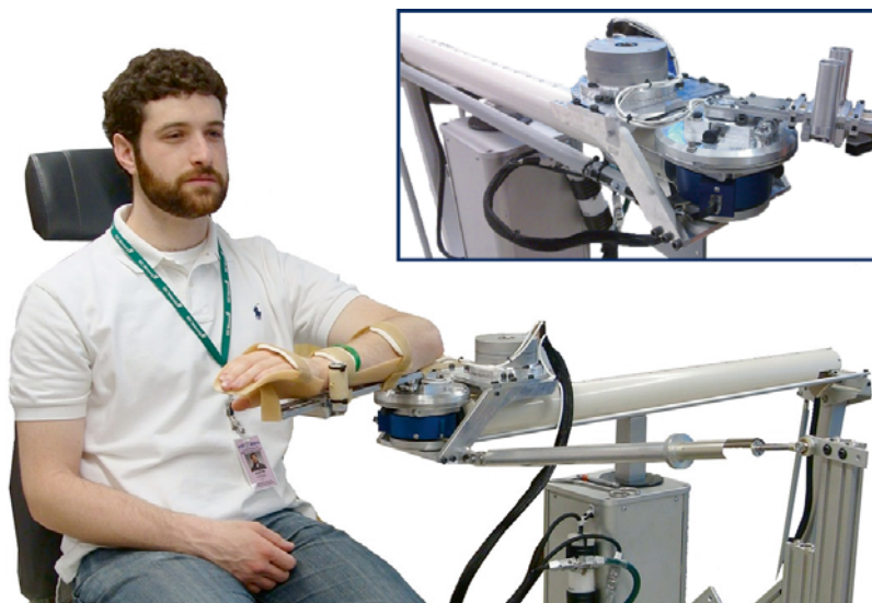
Fig. 18.5 The ACT-2D robotic device allows for single-joint perturbations at the elbow combined with adjustable shoulder abduction loading to study the relationship
