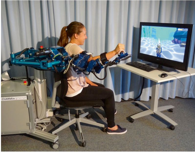
Fig. 17.10 Visualization of a possible setup of ChARMin and the visual interface shown with a healthy subject
