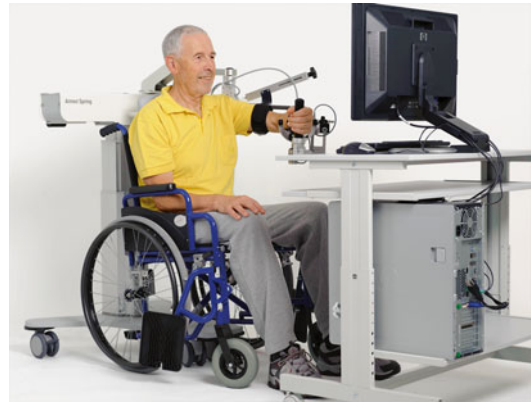
Fig. 27.3 ArmeoSpring, developed by Hocoma AG based on T-WREX, is designed to be more quickly adjustable than T-WREX for easier clinical use (Courtesy Hocoma AG)
