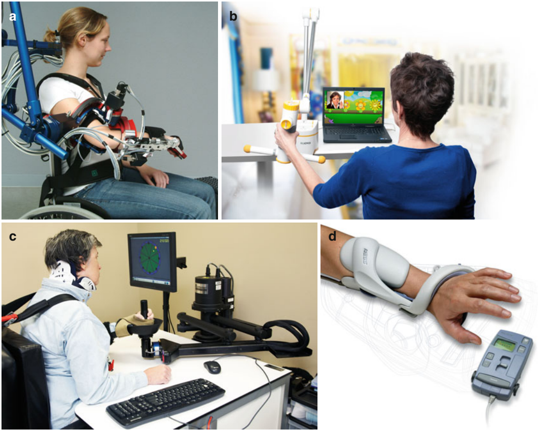
Fig. 7.2 Upper extremity training and assessment devices. This figure shows some devices that are already used for the training of the upper extremity. (a) The ARMinII device (Photo used with permission from Tobis
