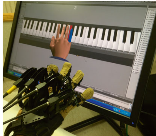
Fig. 28.2 The NJIT-TrackGlove system utilizes a 6-degree-of-freedom magnetic tracker, the TrakStar (Ascension Technology Corporation, USA) and a 22-DOF Cyberglove (Cyberglove Systems, USA). The simulation pictured also utilizes the Cybergrasp, a cable-actuated robotic exoskeleton. In the pictured simulation, the Virtual Piano Trainer, the magnetic tracker allows the participant to position their hand over the virtual keyboard and the Cyberglove allows them to strike keys with a specific finger. The Cybergrasp can be programmed to provide haptically rendered collisions when keys are pressed or assistance in maintaining extension of non-cued fingers for more impaired subjects [106]
