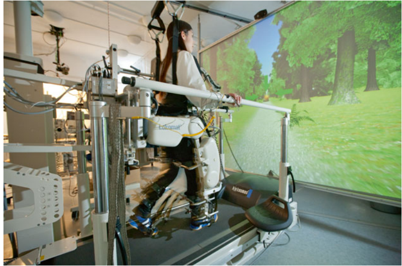
Fig. 19.4 Walking through a virtual environment. Lokomat in combination with a virtual reality back-projection display system
