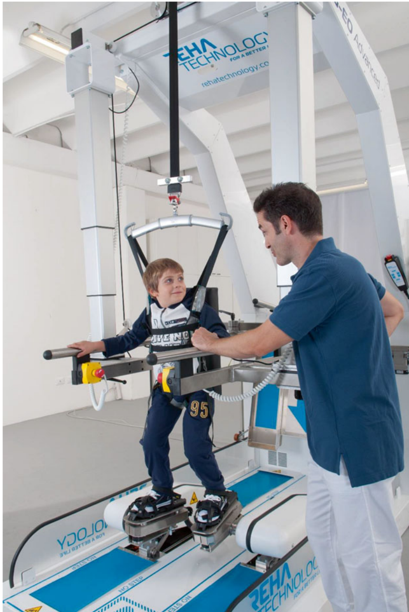
Fig. 14.3 The G-EO System (Reha Technology AG, Olten, Switzerland) is a high-tech end-effector device that allows children and adults to execute a repetitive walking pattern in either a passive, an adaptive-assisted, or adaptive way. Moreover, it can be set to simulate walking up or down the stairs (in the G-EO Evolution). The end-effector
