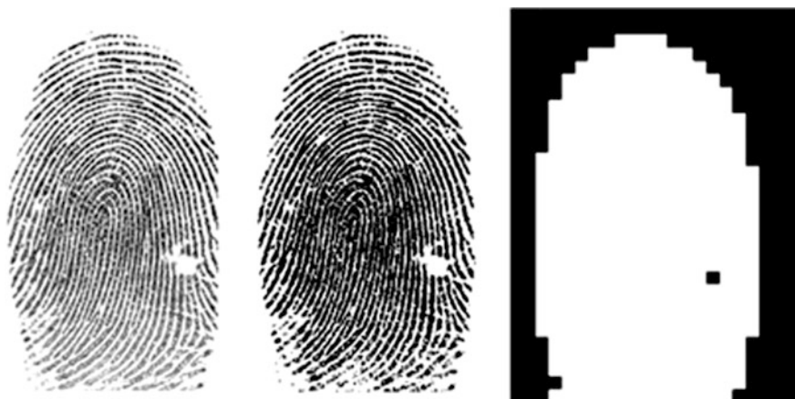
Fig. 3 Steps of preprocessing. From left original image, binarized image, mask ( source own work)
