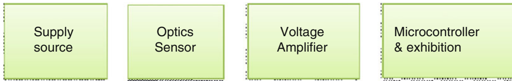
Fig. 29.3 Blocks diagram of the data acquisition system
