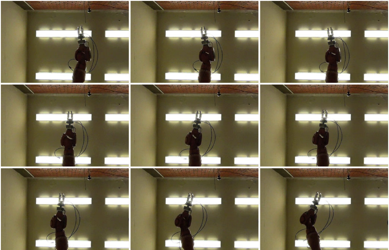
Fig. 28.5 Sequence of movements based on three-dimensional information
