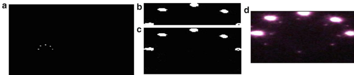
Fig. 14.8 (a) First binarized image. (b) Sub image based on max and min spots coordinates. (c) Sub image (b) double sized. (d) Sub image1. Interest region
