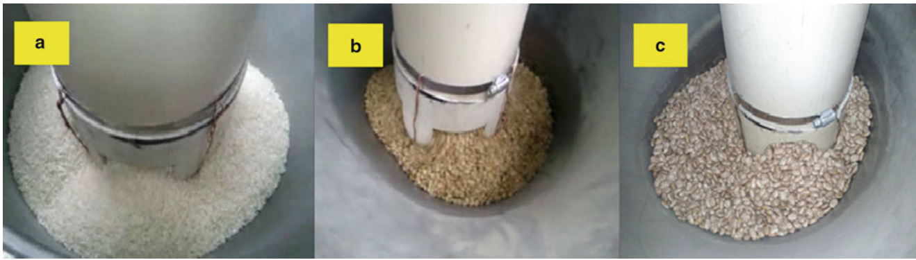
Fig. 33.4 Pilot Testing dispenser, rice (a), chickpea (b) and beans (c)
