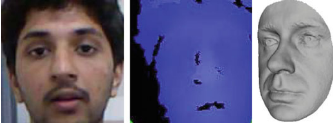
Fig. 12.1 From left to right: traditional 2D color image, depth map captured using Kinect, and traditional 3D image. Images taken from [5, 17]
