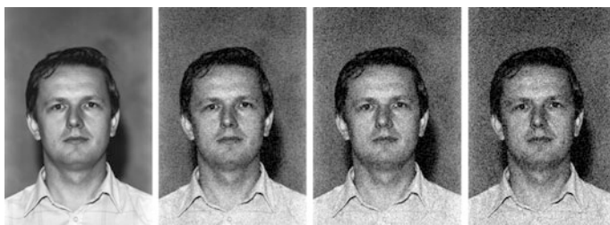
Fig. 6.11 Example of the effects of increasing Poisson noise (decreasing illuminance) on facial images. The upper leftmost image is the pristine input image followed by decreasing illuminance (0.09, 0.06, and 0.04 foot-candles, respectively; note: full moon is approx. 0.02 foot-candles). Images have been contrast-stretched to highlight the effects of the noise
