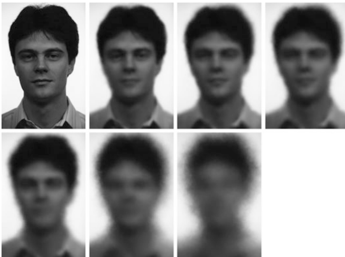
Fig. 6.18 Example of the effects of increasing atmospheric turbulence on facial images. The upper leftmost image is the “pristine” input image followed by increasing turbulence strength ( C_n^2 = 2.5 \times 10^{-14} \text{ m}^{-2/3} , 5.0 \times 10^{-14} \text{ m}^{-2/3} , 7.5 \times 10^{-14} \text{ m}^{-2/3} , 1.0 \times 10^{-13} \text{ m}^{-2/3} , 2.5 \times 10^{-13} \text{ m}^{-2/3} , 5.0 \times 10^{-13} \text{ m}^{-2/3} , respectively)
