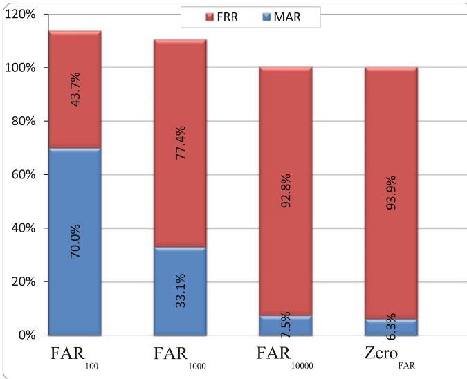
Fig. 9.25 FRR and MAR values computed for Thr_C at different levels of FAR for EyeFace SDK. The computed thresholds are 0.3544, 0.4836, 0.6282, and 0.6472 for FAR_{100} , FAR_{1000} , FAR_{10000} , and Zero_{FAR} , respectively
