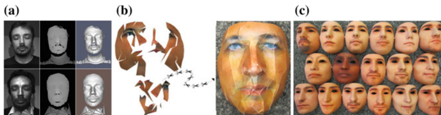
Fig. 8.6 a Example shots from Morpho: The top row shows a real access from a user in grayscale texture (2D), depth map (2.5D), and 3D model format, while an attacker wearing the same users mask is displayed in the bottom . b Example papercraft mask from 3DMAD. c 17 Wearable resin masks from 3DMAD [81]
