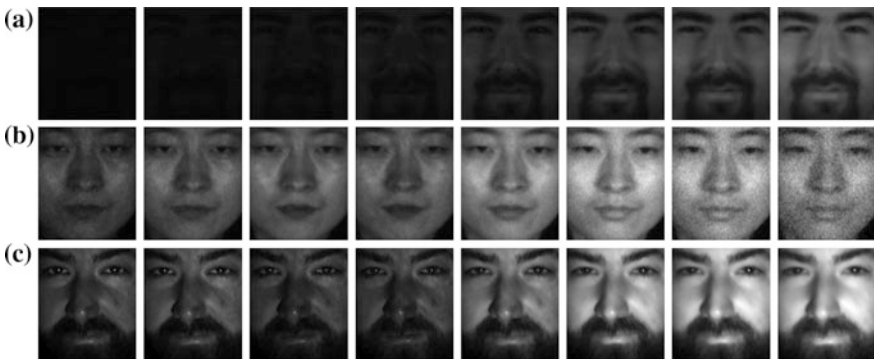
Fig. 3.13 Comparison of three HFDs using LCTFs: (a) the IRIS-M database [21], (b) the PolyU-HSFD [22], and (c) the IRIS-HFD-2014. The HFIs are covered by a range of 480–690 nm in 30-nm intervals. While (a) and (b) were acquired with constant exposure time over the visible spectral range, (c) was acquired with adjusted exposure times
