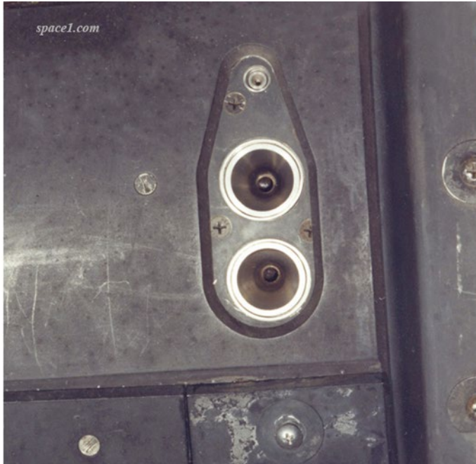
Fig. 13.14 Thrusters installed on the Mercury capsule. (Photo Courtesy of Historic Space Systems)
