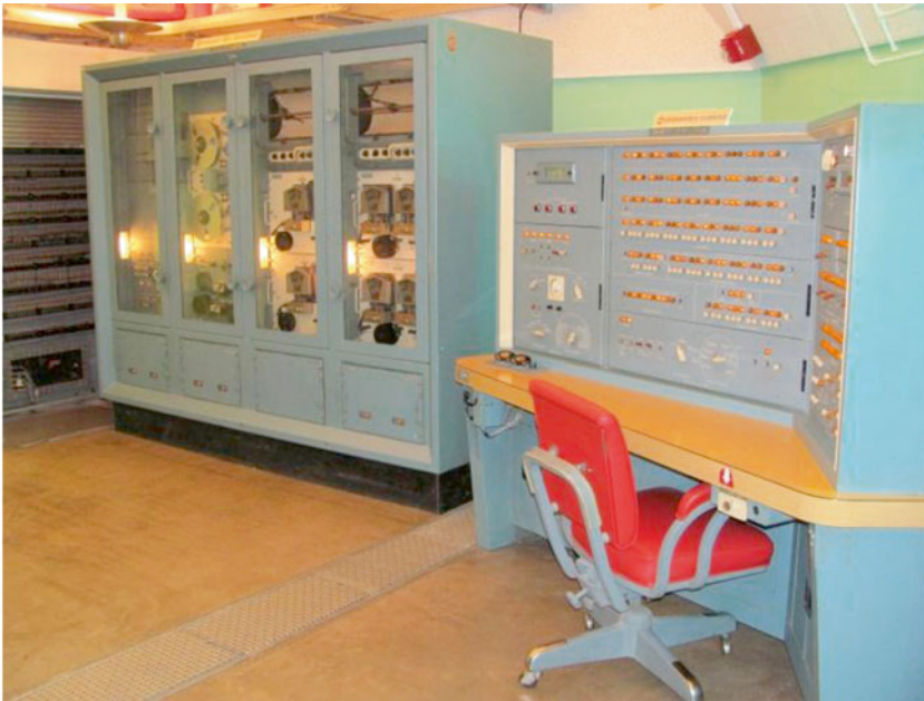
Fig. A.3.7 The GE/Burroughs Guidance Computer. This is the computer that sent commands to the Atlas booster for steering commands. (Photo courtesy of the Air Force Space Museum)
