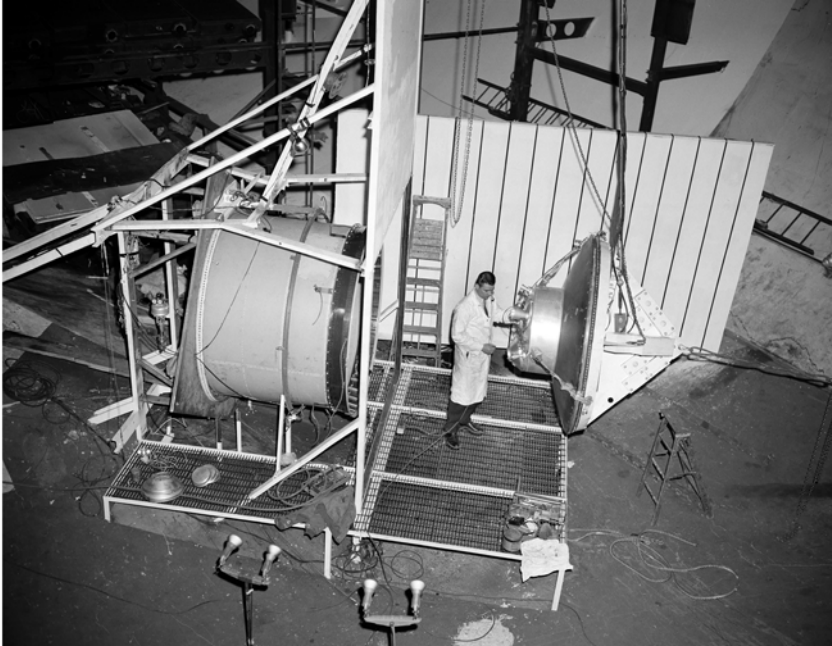
Fig. 7.7 Testing the posigrade rocket separation of the spacecraft from the launch vehicle. (Photo courtesy of NASA)
