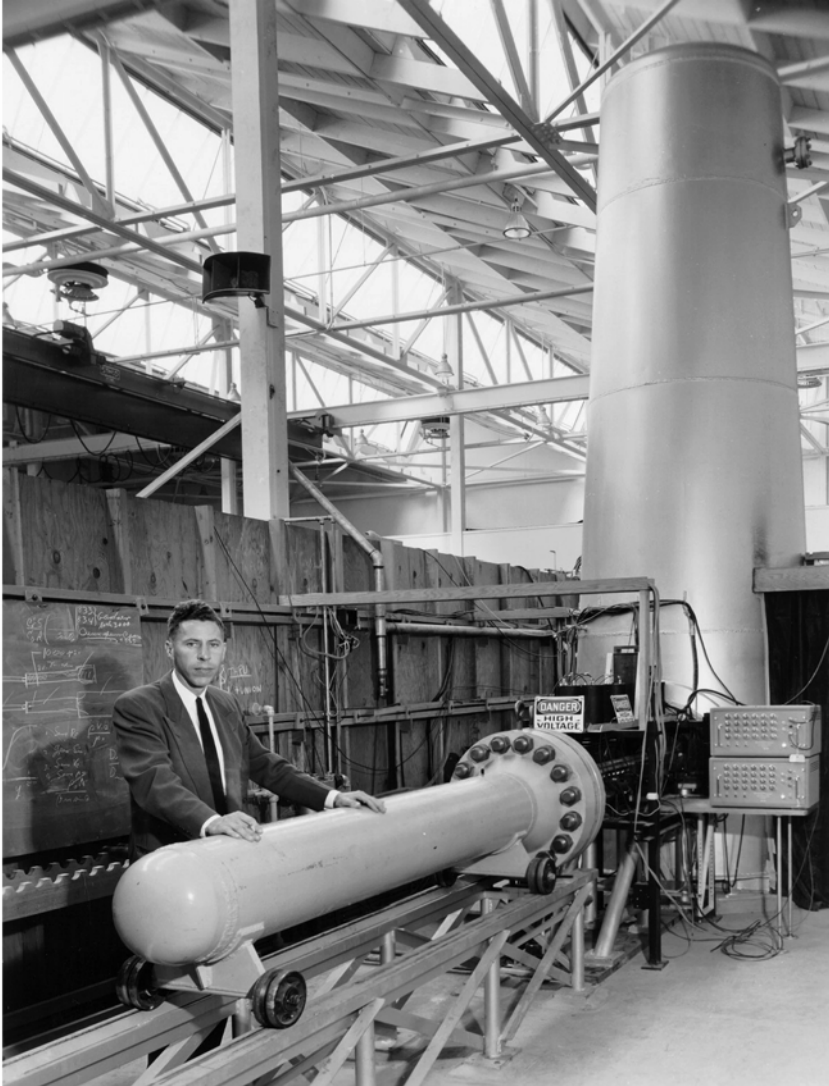
Fig. 7.11 Alfred J. Eggers, Jr. beside the Atmosphere Entry Simulator used on Mercury models. (Photo Courtesy of NASA)
