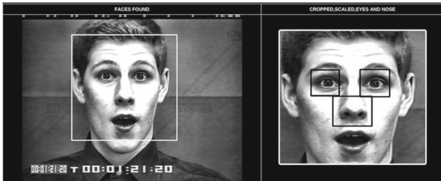
Fig. 7 Face detection, preprocessing, cropping, scaling
