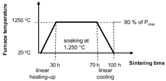
The CBN segments are sintered in a smaller furnace. A total amount of 22 conventional wheels can be stacked including a 5 mm thick spacer between each layer in the larger furnace. The smaller furnace holds 15 layers of superabrasive material segments. Each layer consists of 24 individual segments. In total, an amount of 360 segments can be stacked in the small furnace. This is enough material for nine superabrasive grinding wheels.
