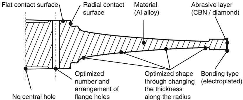
**Fig. 5.1** Design features of high-speed grinding wheels [FERL92, p. 79], with copyright permission by VDI Verlag/Springer Verlag
