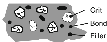
Fig. 3.2 Structure of a resin bonded tool
