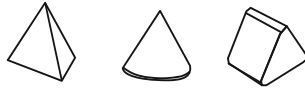
Fig. 4.10 Example shapes of the abrasive particles for vibratory grinding after [ROES12, WALT12]
