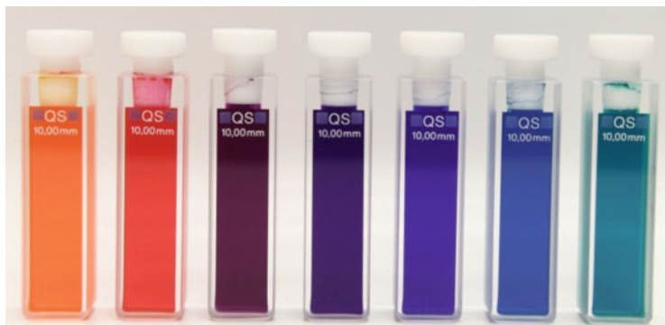
Fig. 2 The optical properties of merocyanine dyes are easily modified by carefully adjusting the strengths of the electron-rich and electron-poor end groups
