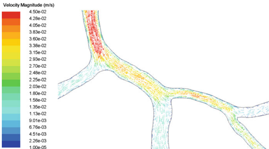
Fig. 13.6 Vector plot of the velocity at junction J_1 , J_2 , and J_3
