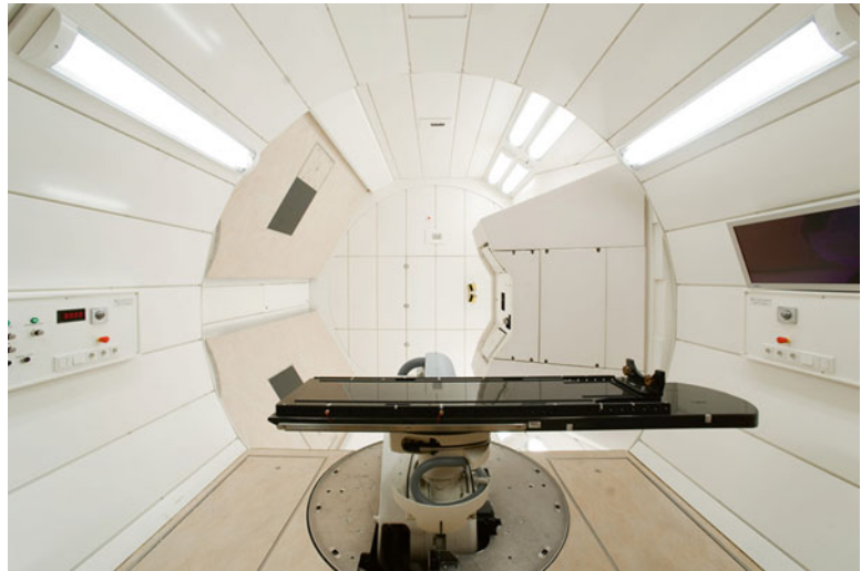
Fig. 5.14 Treatment room adjacent to the gantry at HIT. The possibility to rotate the beam delivery exit and the patient's table gives to the physician a virtually infinity possible number of irradiation field (Universitätsklinikum Heidelberg)
