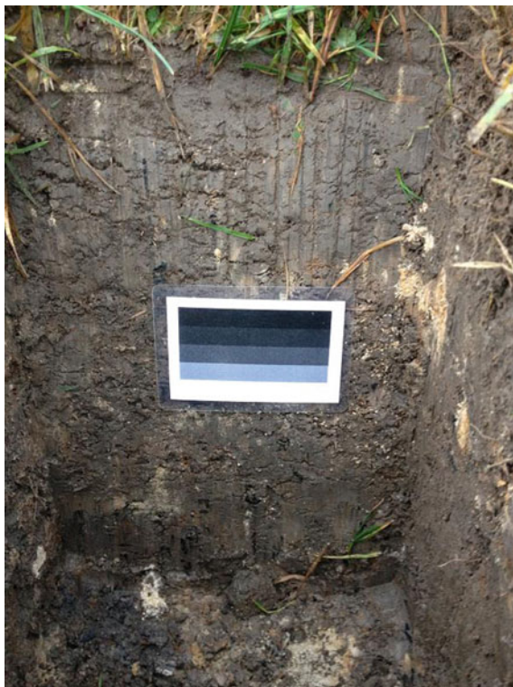
Fig. 7.5 Example of image acquired of topsoil profile for visual soil assessment model
