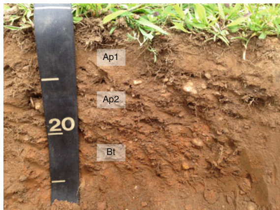
Fig. 26.6 Nixon soil profile for Plot 2 showing an increase in coarse fragments starting around 10 cm, an argillic horizon around 20 cm, and a decrease in root abundance, distribution, and size starting around 10 cm
