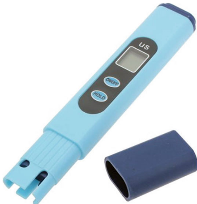
Fig. 15.1 Simple, typical handheld electrical conductivity meter
