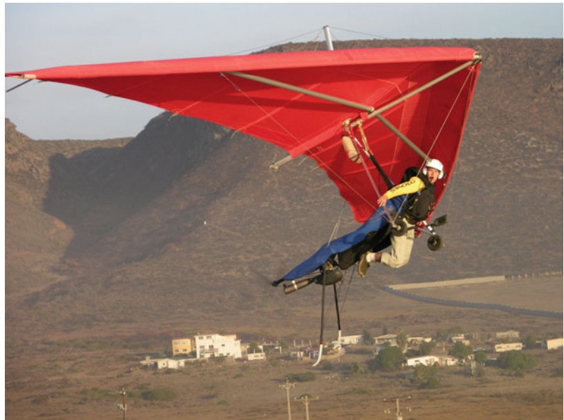
Fig. 17.11 Powered hang glider during takeoff
