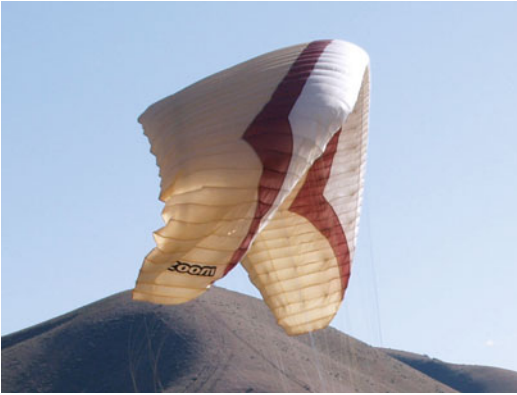
Fig. 17.5 Asymmetrical collapse. In the series by Schulze et al., an asymmetrical collapse (85.1 %) was a more common cause of incidents than a frontal collapse (15.9 %) [20]
