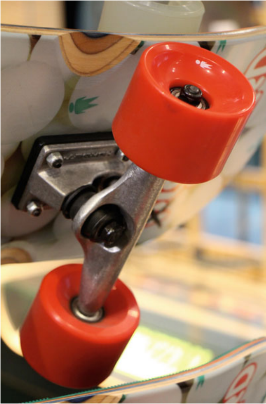
Fig. 14.1 The side of a skateboard with the deck, truck, and wheels (Photo taken with permission at Railside Skateshop, Frankfurt/Main, Germany)
