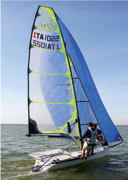
Fig. 22.4 49er is the two-handed skiff-type high-performance Olympic Class. It is powered by a main sail, jib, and 37.16 m 2 triradial asymmetric spinnaker, and both of the crew members are equipped with their own trapeze. The class has been in every Olympic Games since its debut in Sydney, 2000 (Photo: Davide Casadio)
