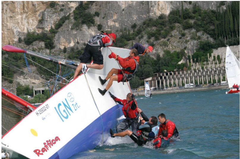
Fig. 22.3 Open class “Raffica” at the Centomiglia del Garda regatta, Lake Garda, Italy. The boat capsized due to the breakage of the keel (Photo: Davide Casadio)
