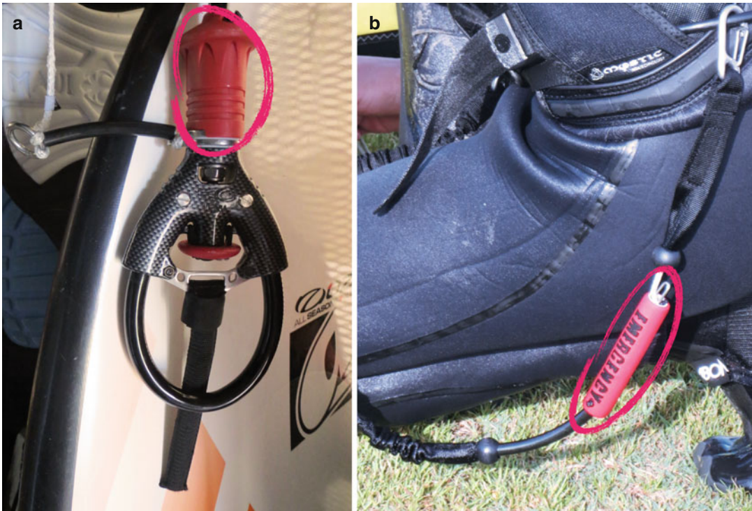
Fig. 15.3 Safety systems. The chicken loop is fitted with a rapid-release system (a), allowing the kiter to immediately detach himself from the kite in the event of an incident. This causes the kite to deflate and lose power. A
