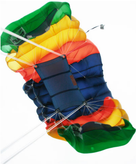
Fig. 19.1 Operation of the slider
