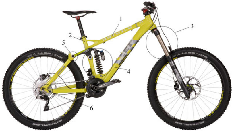
Fig. 12.4 1 top tube (length, 560–620 mm); 2 seat tube (430–480 mm); 3 front suspension; 4 rear suspension; 5 upper linkages consisting of two wheel articulations which act in one axis; 6 regarding the suspension centers of rotation on each side absorb the bumpiness of the area additionally
