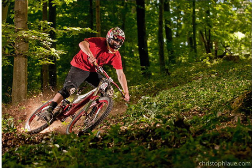
Fig. 12.2 A compact and low frame with a low bottom-bracket height gives the downhill biker the best possible traction and an easy handling while riding at high velocities (Photo courtesy of Felix Weilbach)
