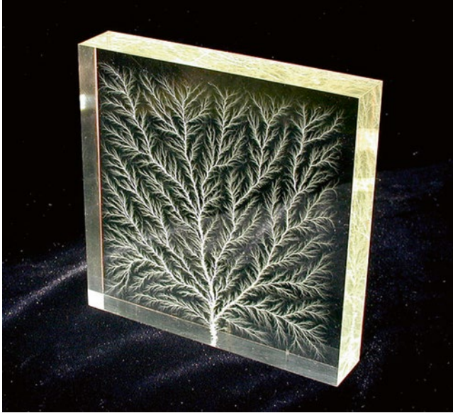
Fig. 5.4 Profile of electrical trees in PMMA
