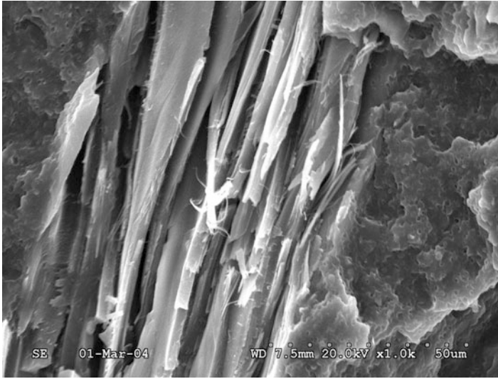
Fig. 17 SEM micrograph showing the fracture of a wood particle during the deformation of PP/wood composites. Good adhesion of the components was achieved by the use of functionalized PP
