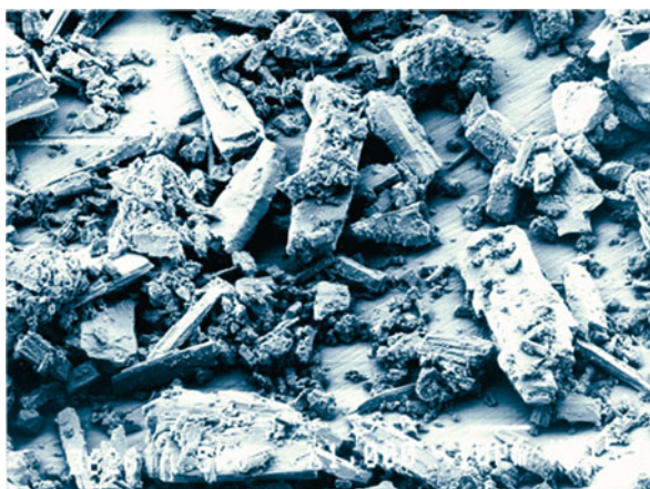
Fig. 2 Scanning electron micrograph: micronized LAR wollastonite flour (magnification 1:1,000)
