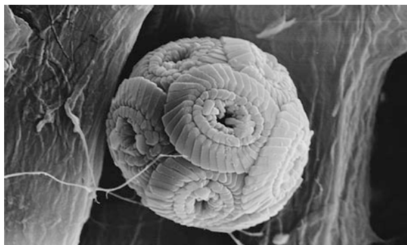
Fig. 1 An SEM image of a coccolith microfossil from a UK chalk deposit – each individual calcite crystallite making up the spherical body is around 3 \mu\text{m} in dimension
