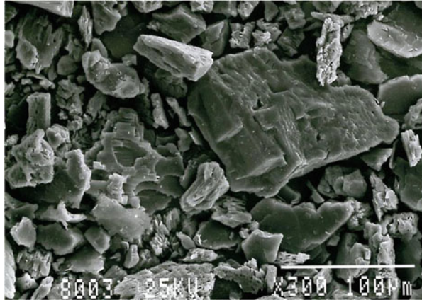
Fig. 3 SEM of feldspar flour: 87% orthoclase, 7% albite, 4% kaolinite, and 2% quartz
