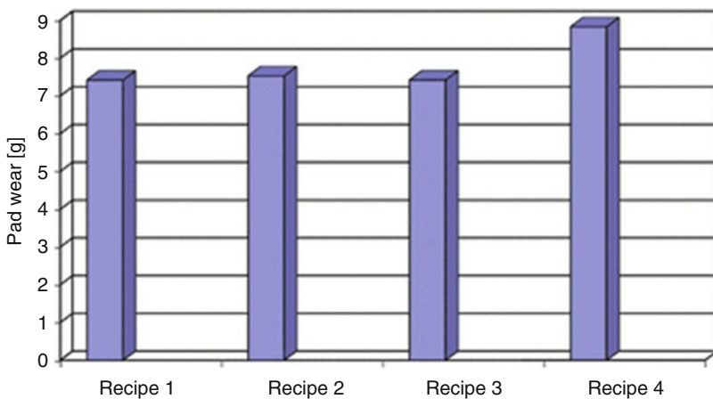
Fig. 14 Pad wear in g of the recipes investigated
