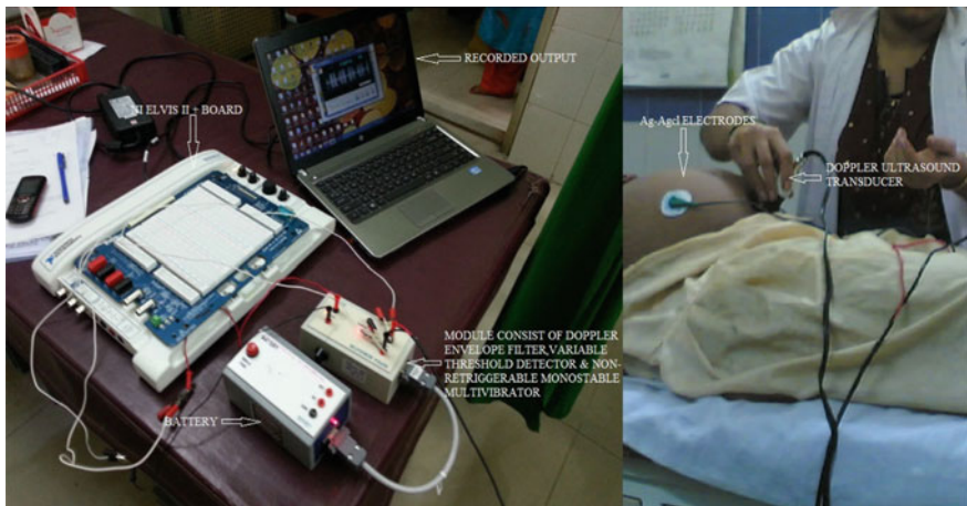
Fig. 2 Real time abdominal Doppler ultrasound recording setup in hospital
