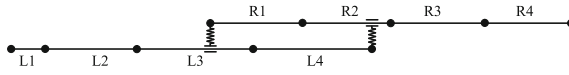
Fig. 12 Element numbering of the bending flexible hydraulic cylinder. The slides are positioned such that they appear during the highest stresses
