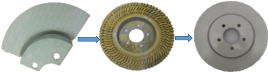
Fig. 4 Assembly process of the disc brake
