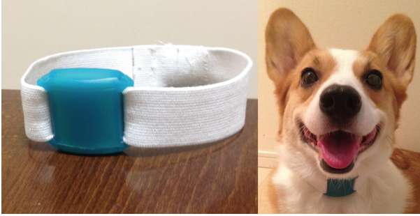
Fig. 12. The appearance of the sensor and how the dog wears it.
