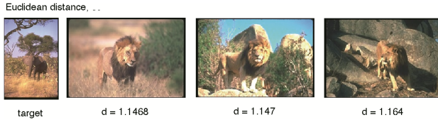
Fig. 5. Top three results for multimodal image retrieval using the target query image (left) and keyword “lion”, using GIST descriptor with Euclidean distance measure for content-based ranking.
