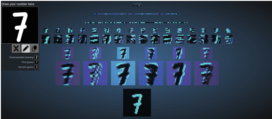
Fig. 1. The proposed visualization: an interactive node-link diagram of a convolutional neural network trained to recognize handwritten digits. On the left is a drawing pad, where the user can draw numbers for the network to classify. The activation level of each node is encoded in hue and brightness. Studying the architecture of the network, and experimenting with its input-output process, can enlighten students of machine learning as to how the network performs its abstraction from images to digits.
