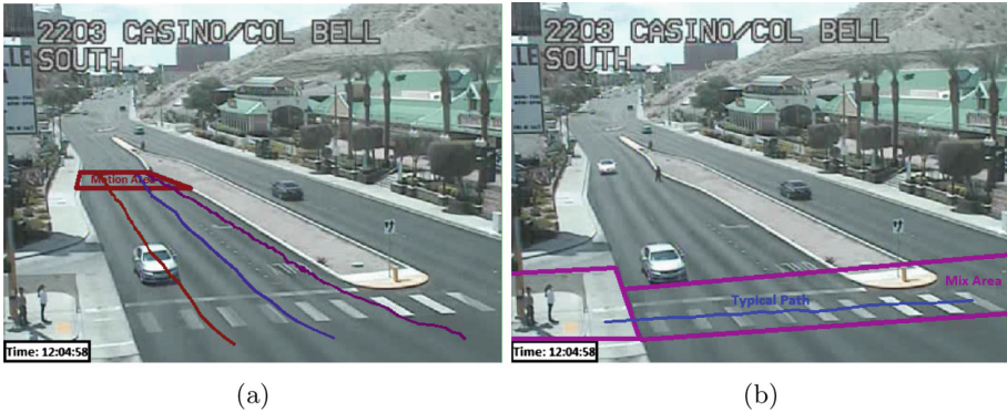
Fig. 1. Defining areas (a) Motion area for vehicle detection (b) Mix area for pedestrian detection through contextual fusion
