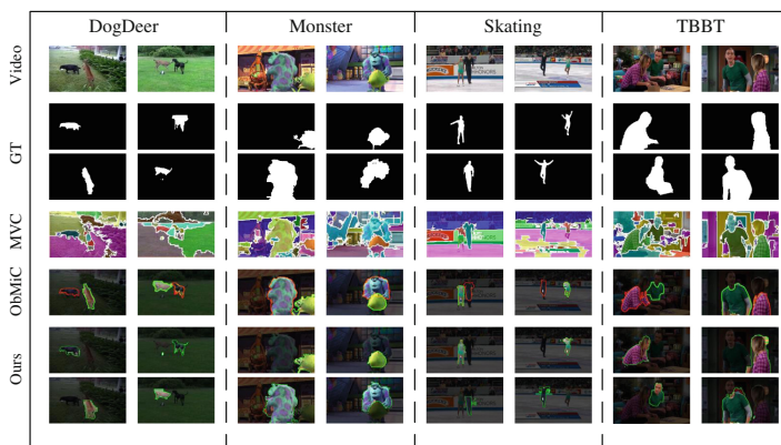
Fig. 8. Multiple objects co-segmentation results on ObMiC dataset. First row is the sample frames of given videos; second row represents the ground truth; from the third to fifth row are the segmentation results from MVC [6], ObMiC [7] and our framework, respectively.
