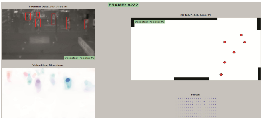
Fig. 8. Ortho-mapping of the detected individuals and their crowd properties from thermal sensors onto Athens international airport terminal plan.
