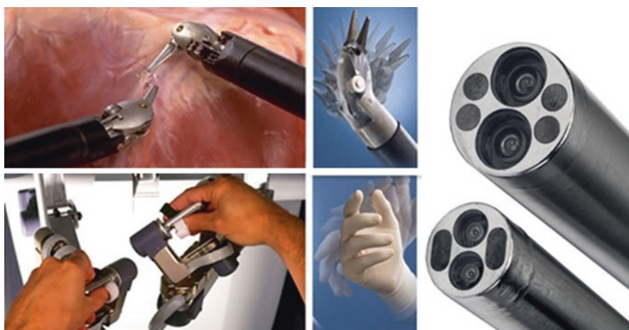
Fig. 11.9 Surgeon manipulates the joysticks operating the EndoWrist instruments that have a range of motion comparable to the human risk motion. The two-lens robotic scopes that provide a fantastic high-definition three-dimensional view
