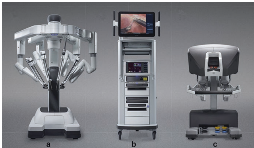
Fig. 11.8 Da Vinci Xi System. (a) Patient side cart. (b) 3D vision recorder. (c) Surgeon control console
