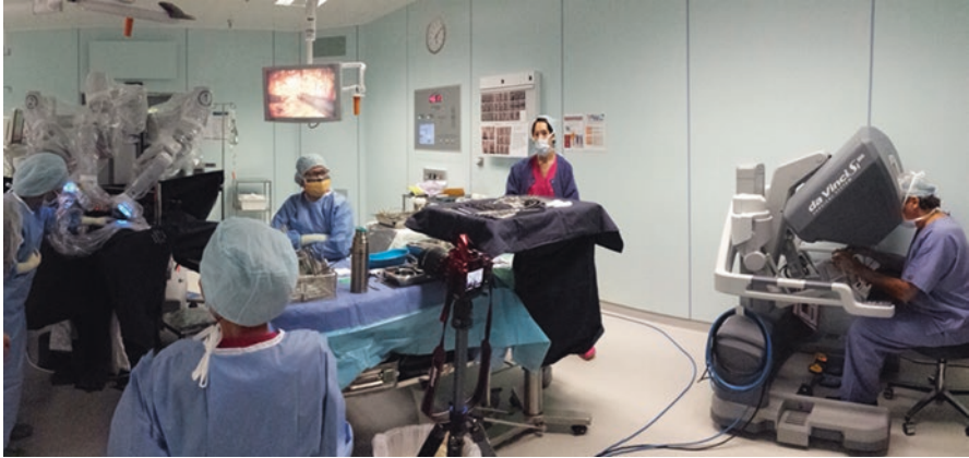
Fig. 11.16 Surgeon seated at the robot console distant about 4–5 metres from the patient, operating the robot arms and camera with joysticks and pedals
