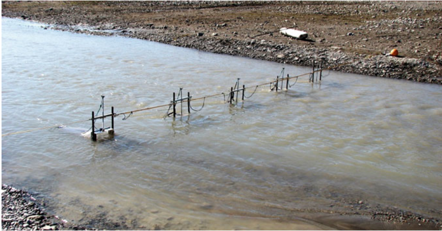
Fig. 2 Example measurement profile comprising RBT devices (5 modules) with the securing system
