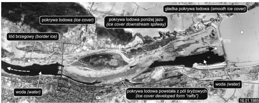
Fig. 4 Aerial photo of the ice forms downstream of Włocławek Dam on January 16, 1985 (courtesy of Prof. M. Grześ)
