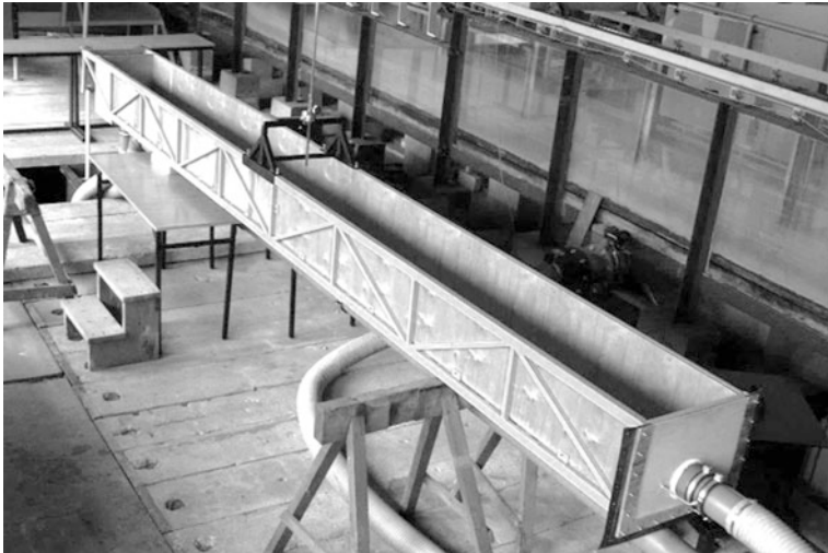
Fig. 6 Photograph of laboratory stand for surface and sewage flow interaction experiments
