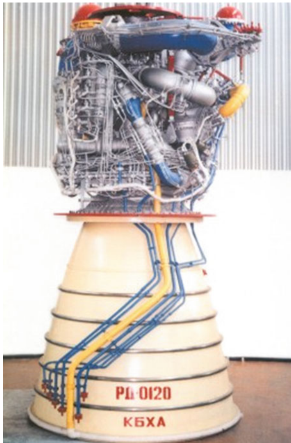
Fig. 8 Cryogenic high-pressure staged combustion engine RD-0120
