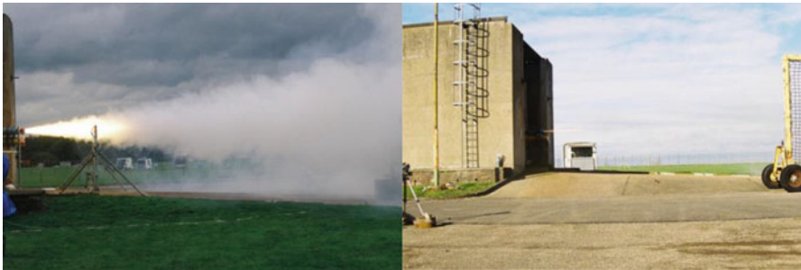
Fig. 3 Experimental firings. The motor firing on the left is a typical composite motor, while that on the right is an experimental composition of the same performance, but smokeless. This was part of a multinational program involving the United Kingdom, France, Germany, and the United States [7]
