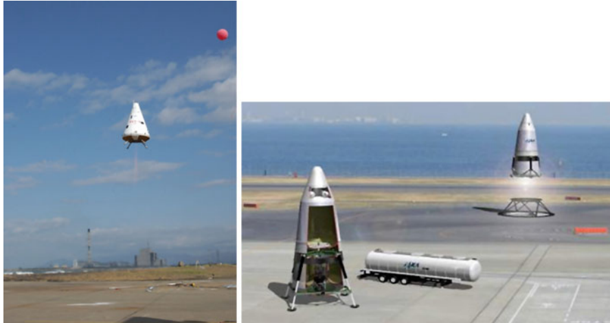
Fig. 13 Flight test of RVT (left) and image of reusable sounding rocket (right)
