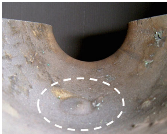
Fig. 4 Buckling of PSZ top coat induced by compressive stress state
