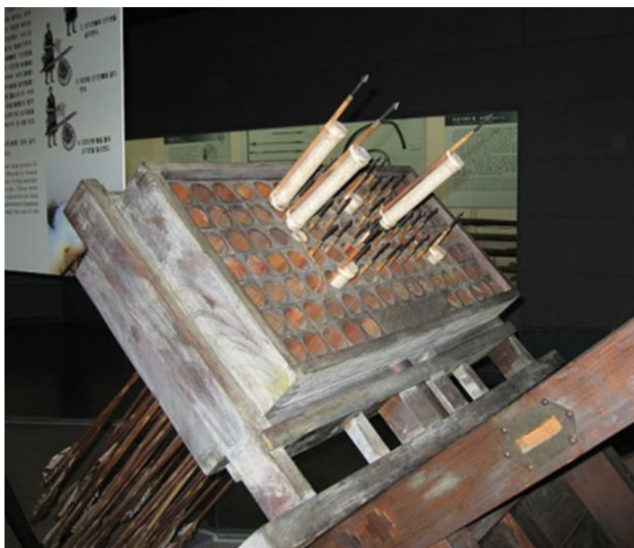
Fig. 7 Korean multiple launcher “hwacha” as displayed at the War Museum, Seoul, Korea
