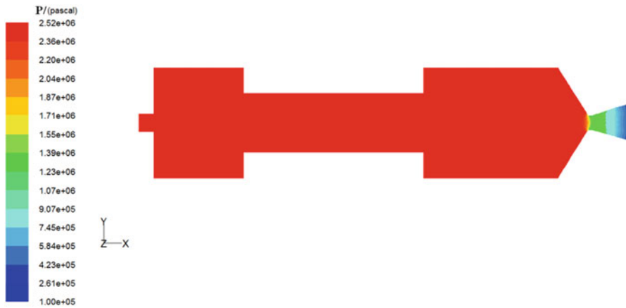
Fig. 13 The pressure distribution of hybrid engine with steady calculation
