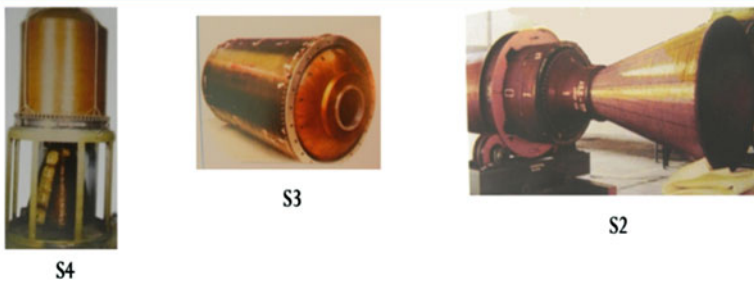
Fig. 3 SLV-3 solid stages description
