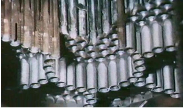
Fig. 17 Baffle arrangement inside an RD-170 chamber
