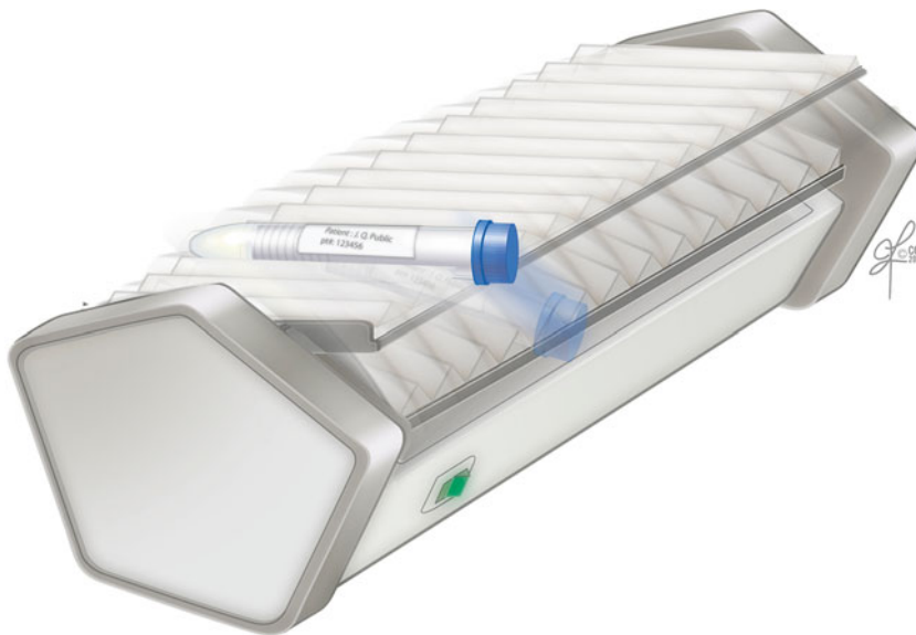
Fig. 9.2 Sample placed on a test tube rocker for 5 min after the addition of Test-Yolk Buffer
